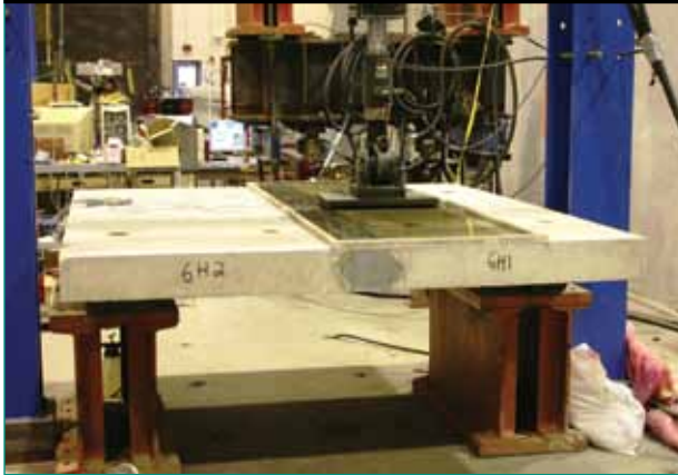
Figure 3. Field-cast UHPC longitudinal connection cyclic test setup.
