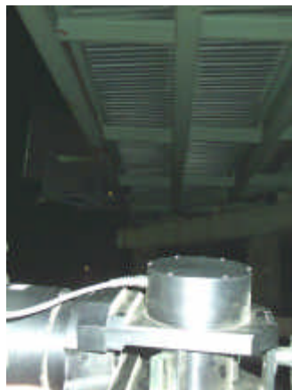
NDEVC laser scanner collecting measurements during the load test.
