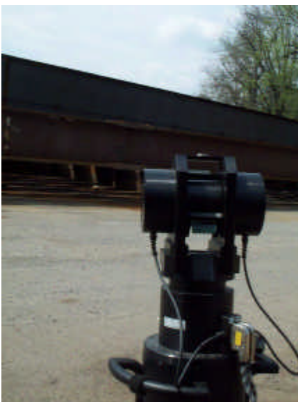
Laser system scanning a fabricated girder.
