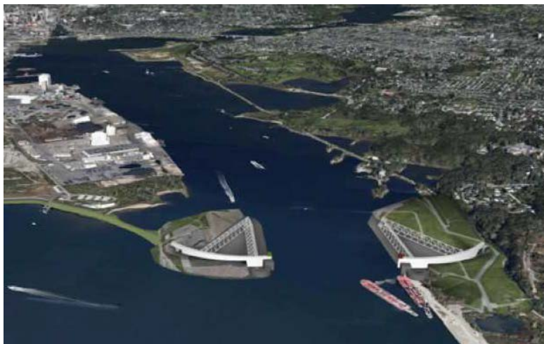
Figure 8: This computer-generated image depicts the placement of a new hurricane barrier design concept that would protect the Port of Providence from a 21-foot storm surge. (Image courtesy of the University of Rhode Island)
