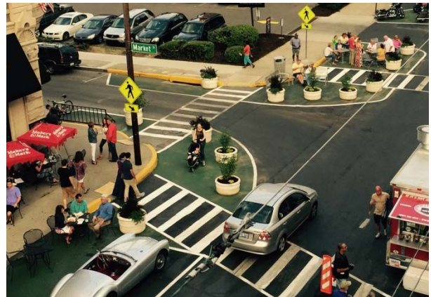
Figure 5: Lexington, Kentucky improved pedestrian safety by painting street space green, which has slowed traffic and shortened pedestrian crossings.
