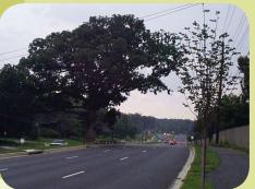
The alignment of a road widening in Maryland was set to run straight through an established oak tree. To preserve the tree, the team realigned the roadway with the tree in the median, redesigned the profile to preserve the tree's root
