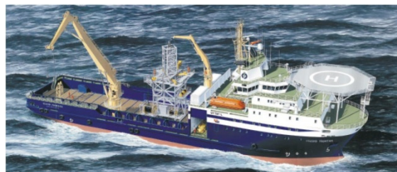
The UT737L tasks include wire-lining operations and deploying a subsea lubricator
