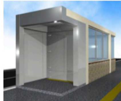
Install water sealing gate on existing structure to make a total protection. Apertures on side walls are covered by reinforced glass.
