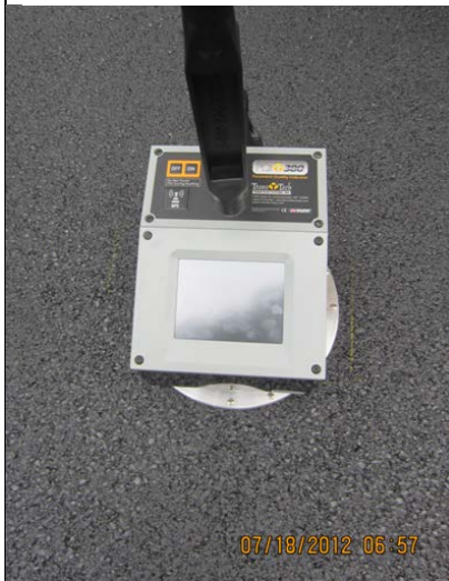
16a. Troxler nuclear density gauge used to monitor the mat density during the rolling operation.
