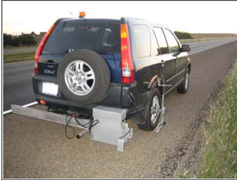
Figure 30. High-speed inertial profiler mounted behind the test vehicle.
