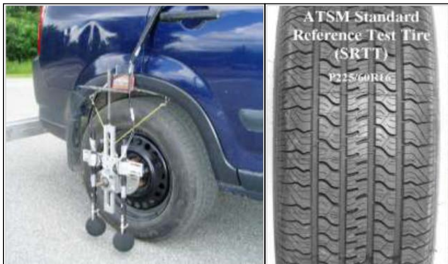
Figure 33. OBSI dual probe system and the SRTT.
