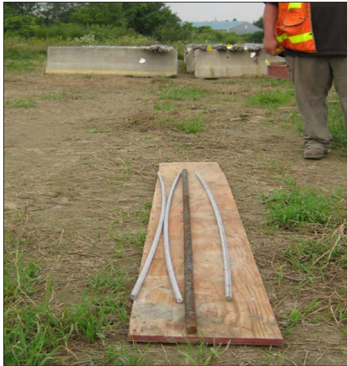
Figure 22. Curved condition of stainless steel rebar.
