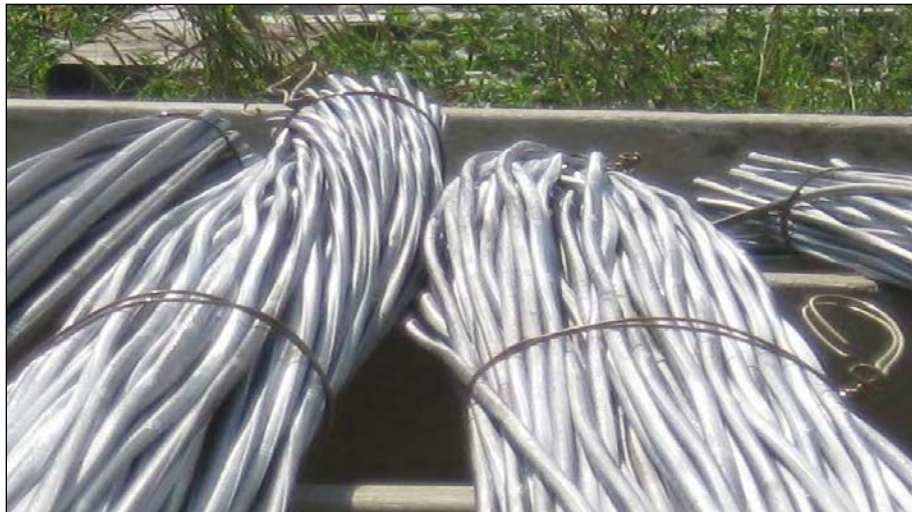
Figure 20. Condition of stainless steel rebar upon arrival.
