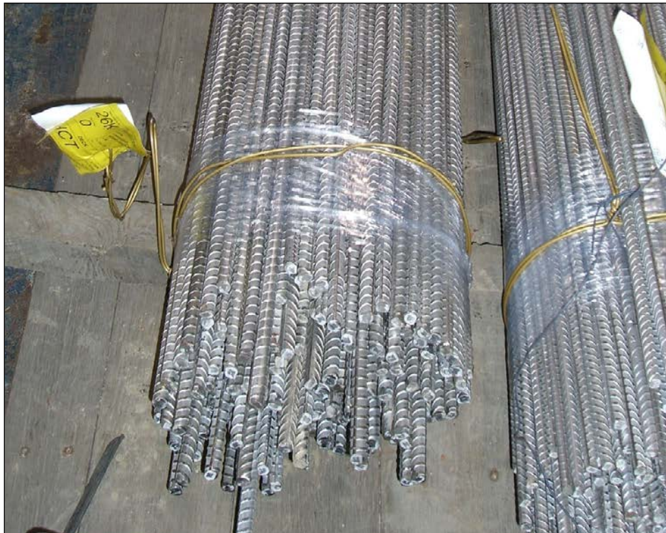
Figure 23. Stainless steel reinforcing bars prior to placement.
