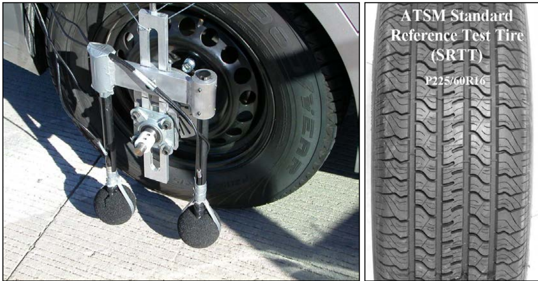
Figure 28. OBSI dual probe system and the SRTT.
