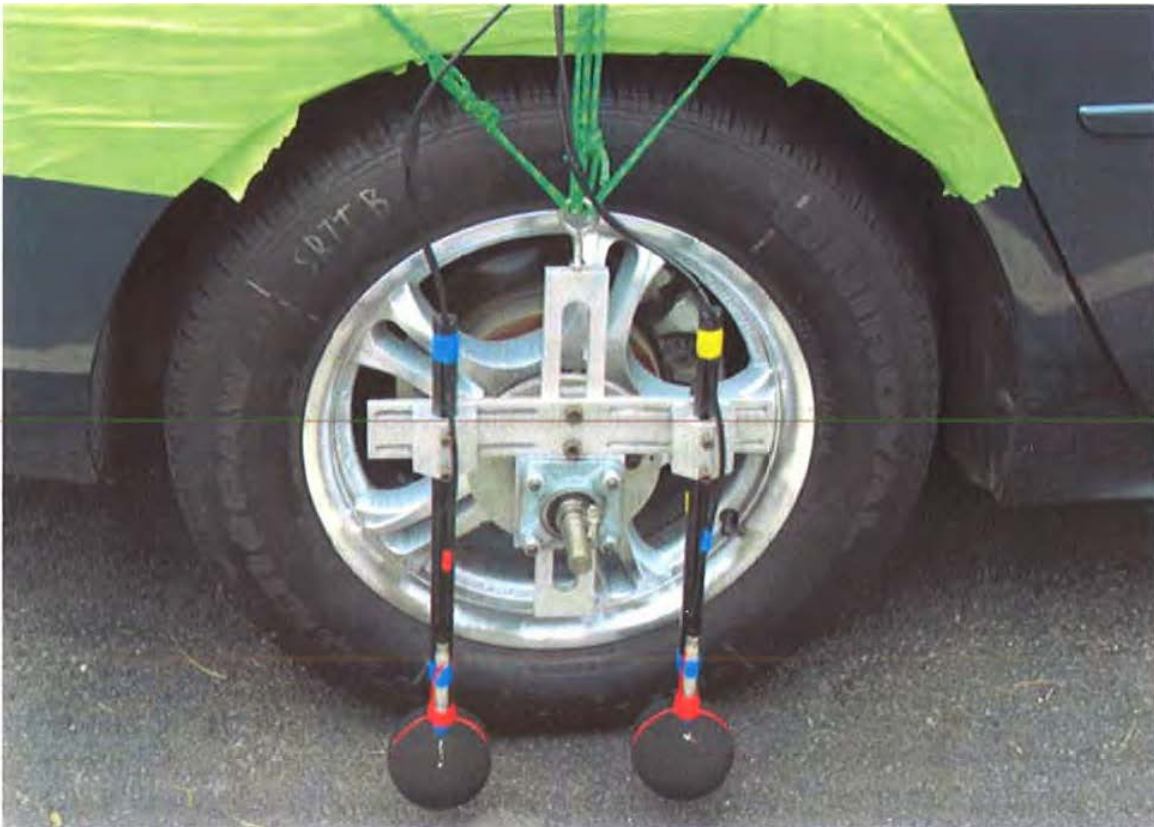
Figure 8. Photo. OBSI dual probe system and the SRTT.
