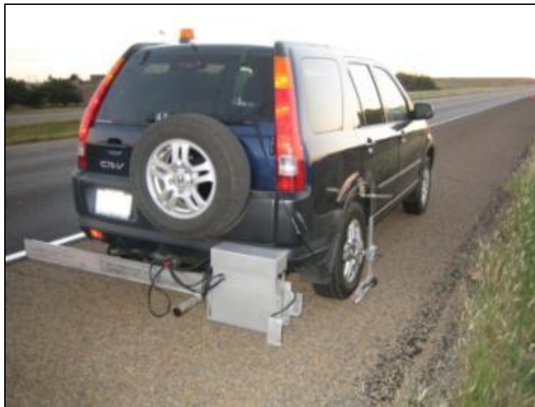
Figure 70. High-speed inertial profiler mounted behind the test vehicle.
