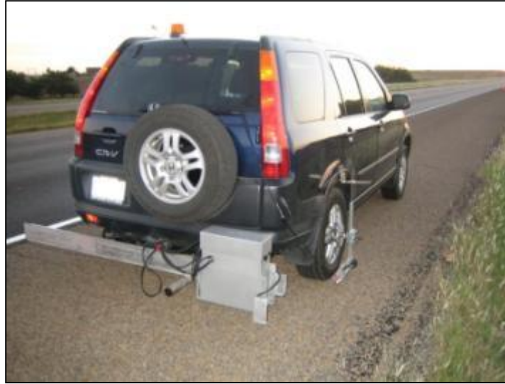
Figure 15. Photo. High-speed inertial profiler mounted behind the test vehicle.
