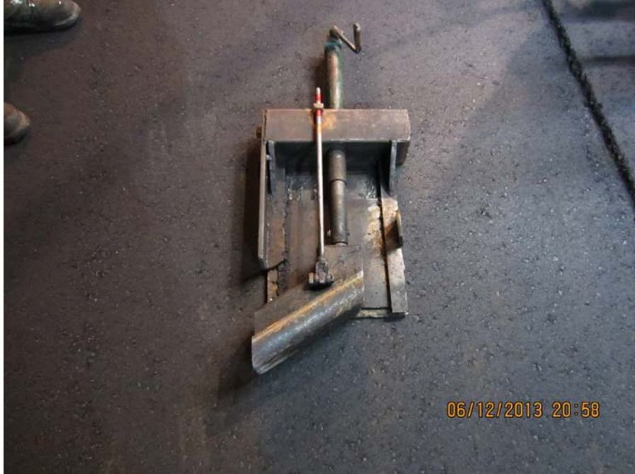
Figure 9. Photo. Contractor's self-manufactured Safety Edge device.
