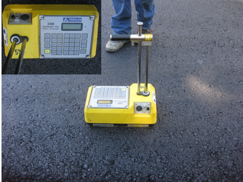
Figure 42. Measuring HMA mat density with a nuclear density gauge on Mountain Ranch Road.
