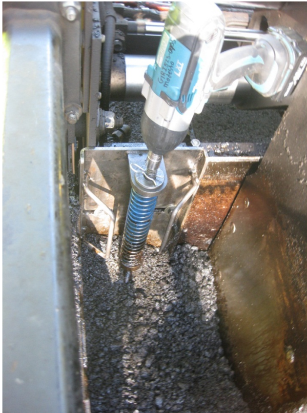
Figure 17. The Safety Edge shoe of the Advantedge® can be raised and lowered by turning the bolt at the top of the device.
