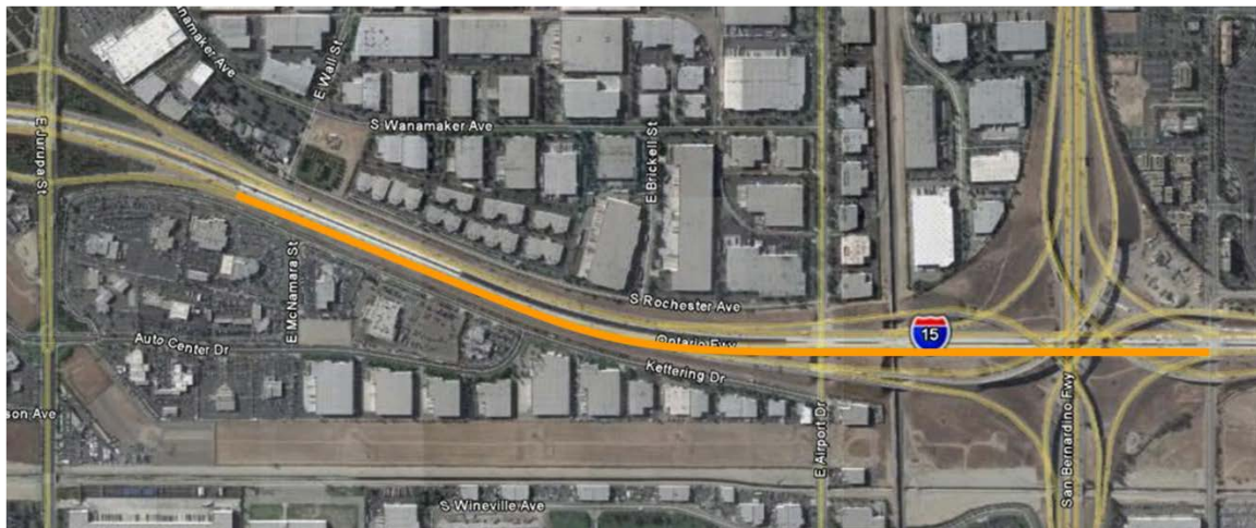
Figure 6. Alignment of roadway that received PCPS slab installation, with horizontal and vertical curves included in the alignment.
