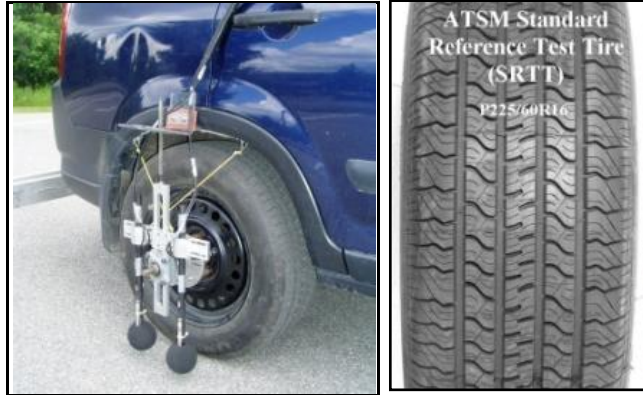
Figure 22. OBSI dual probe system and the SRTT.
