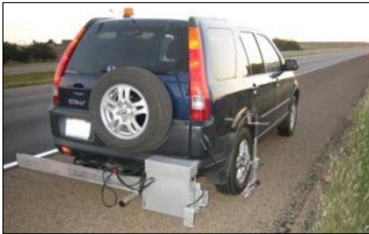
Figure 24. High-speed inertial profiler mounted behind the test vehicle.
