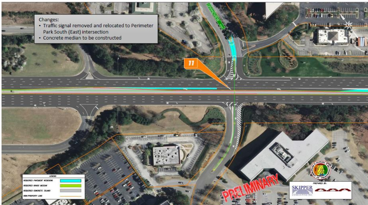
Figure 12. Annotated photo. Work completed on US 280 at Grandview Parkway (courtesy ALDOT).
