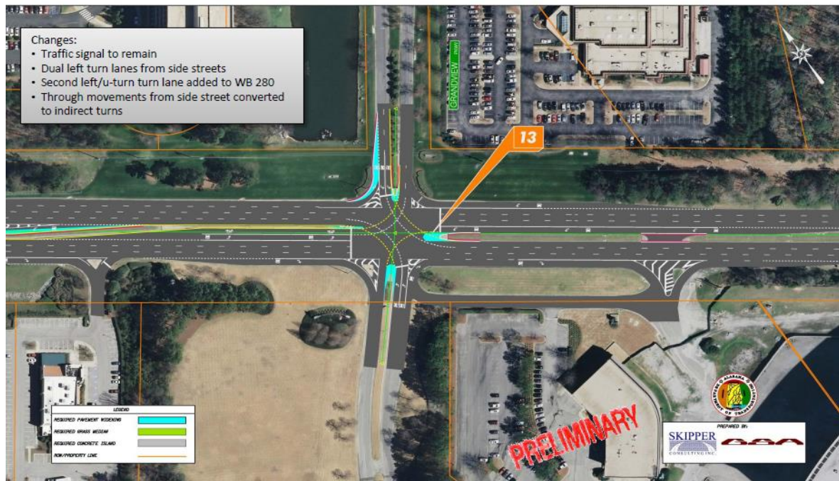
Figure 14. Annotated photo. Work completed on US 280 at Grandview Parkway (East) (courtesy ALDOT).
