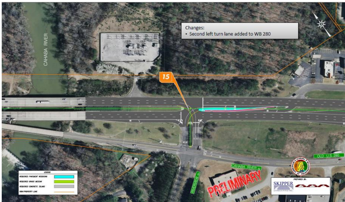
Figure 16. Annotated photo. Work completed on US 280 at Riverview Road (courtesy ALDOT).
