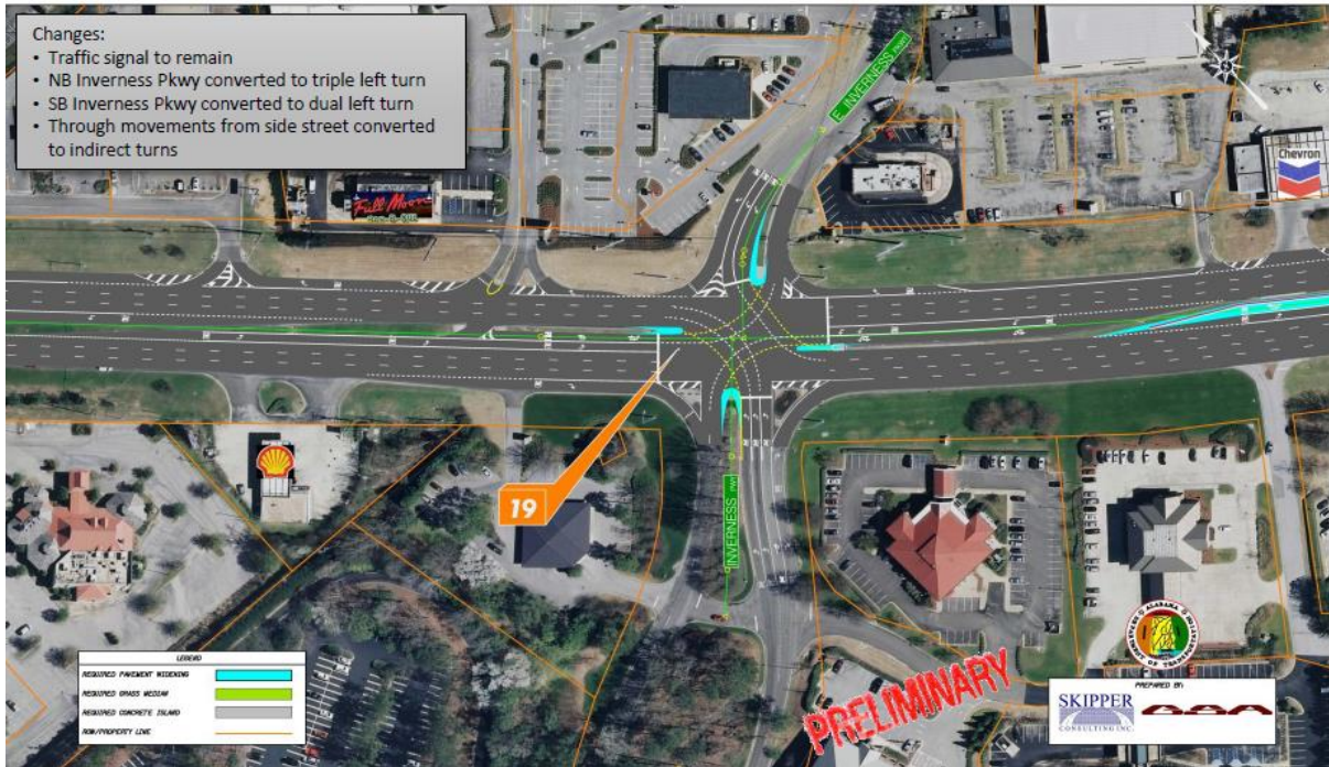
Figure 19. Annotated photo. Work completed on US 280 at Inverness Parkway (courtesy ALDOT).
