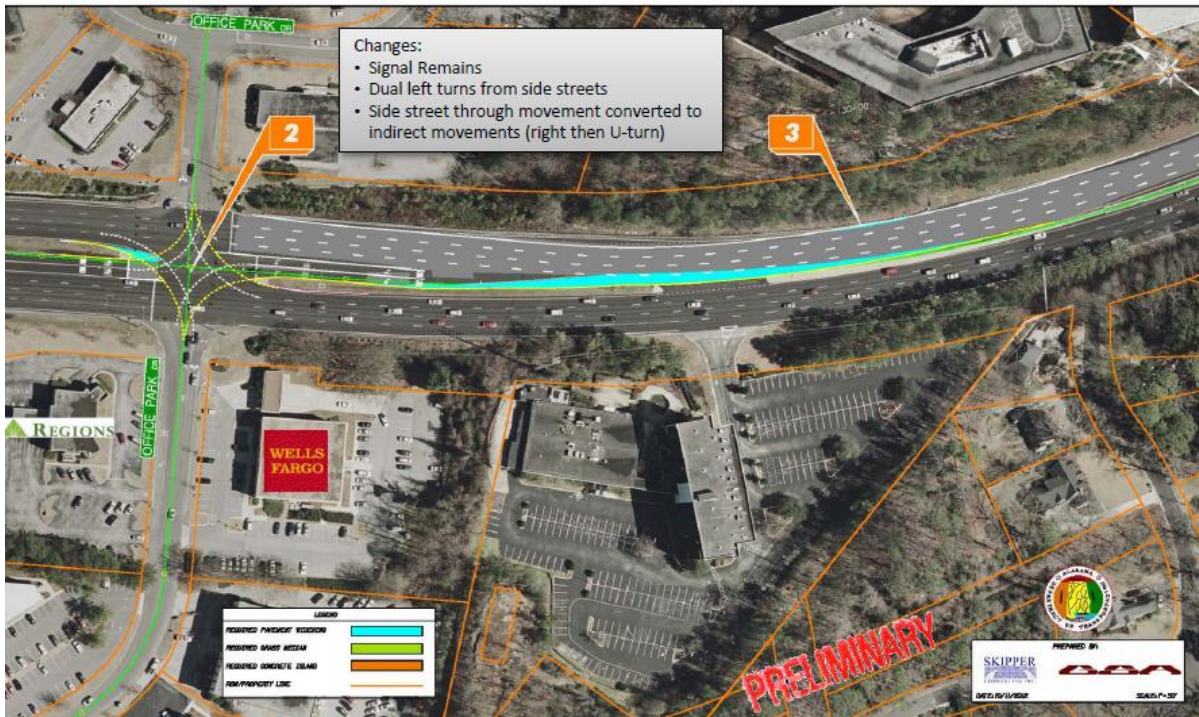
Figure 5. Annotated photo. Work completed on US 280 at Office Park (courtesy ALDOT).
