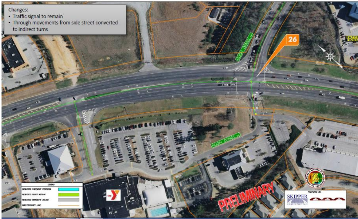
Figure 25. Annotated photo. Work completed on US 280 at Hugh Daniel Drive (courtesy ALDOT).
