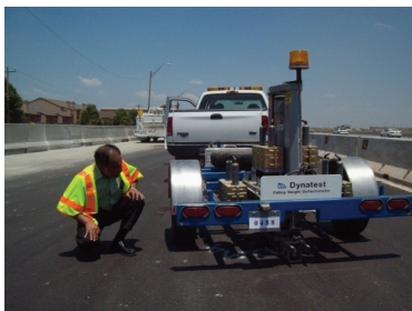
Verifying the seating and location of the test site.
