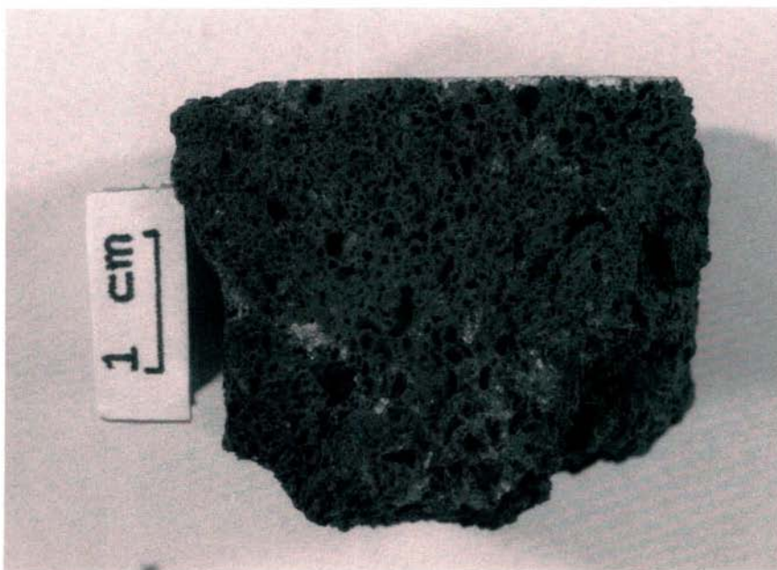
Figure 34. The Rock Basalt (vesicular)
