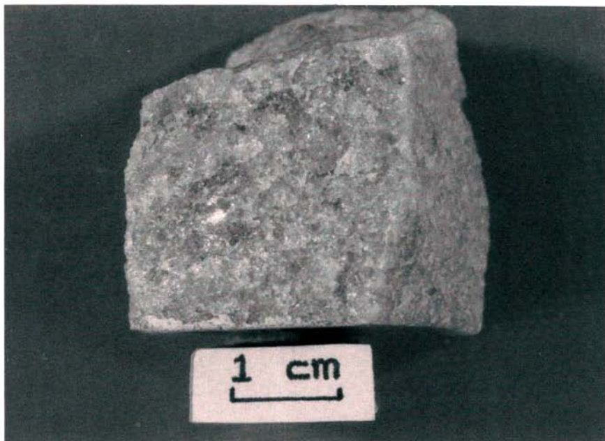
Figure 25. The Rock Quartzite (note more glassy, sharper surface than sandstone)
