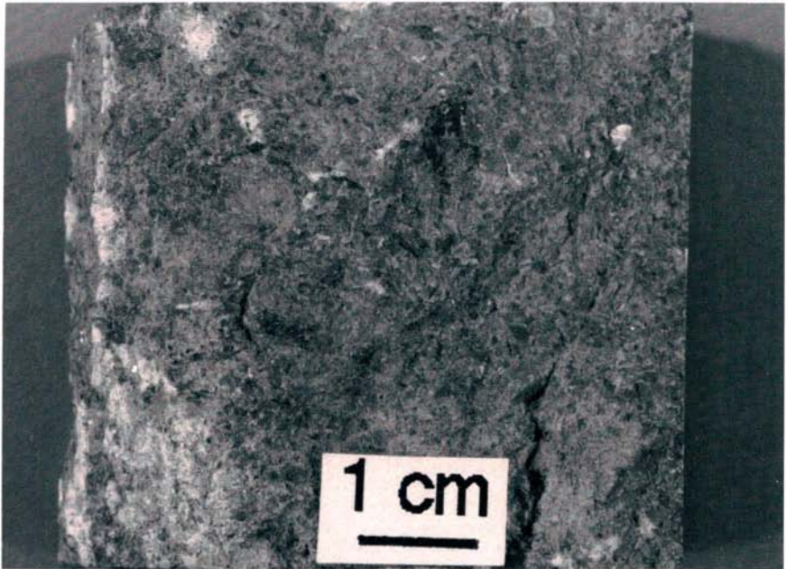
Figure 11. The Rock Limestone (coarse grained example)
