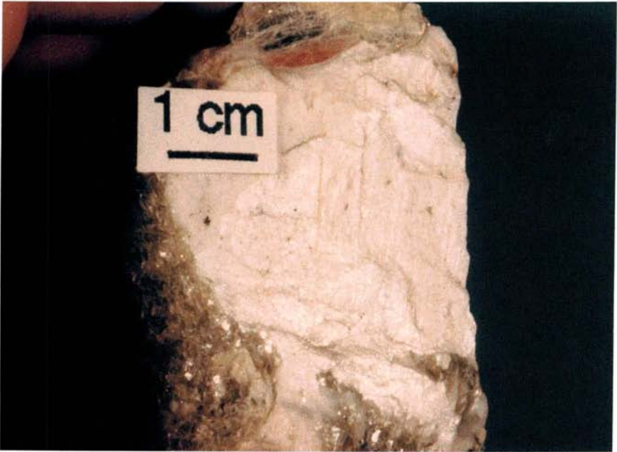
Figure 4. The Mineral Plagioclase (note striations due to crystal structure)
