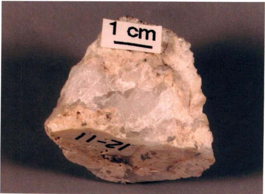
Figure 5. The Mineral Orthoclase (pinkish-tan) and Quartz (white)
