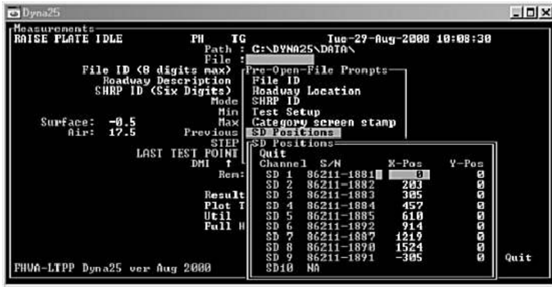
Figure G-1.11 Pre-Open-File Prompts - Check Sensor Position
