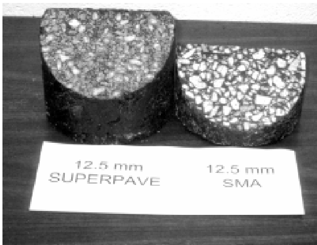
The difference in aggregate structure between dense-graded and SMA is shown in these core samples.
