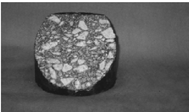
A core sample of 25.0 mm shows a dense-graded mix.
