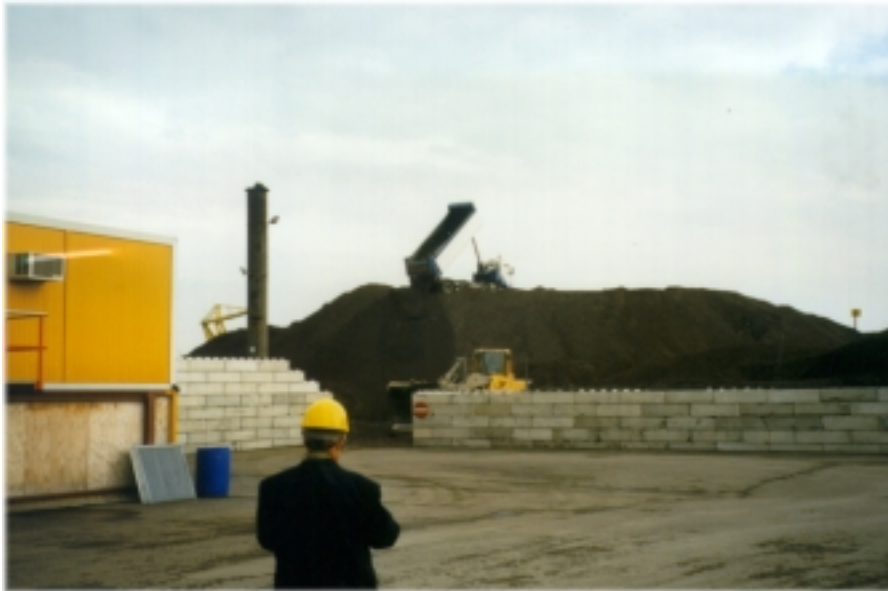
Figure 22. RAP is used at high substitution levels at the Swiss-designed Ammann double drum hot recycling asphalt plant in the Netherlands.
