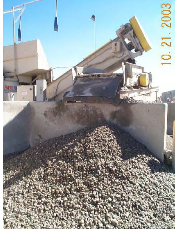
Figure 26. Reclaimed PPCC Coarse Aggregate. Red-I-Mix Concrete Inc. Facility Visit. Irwindale, CA
