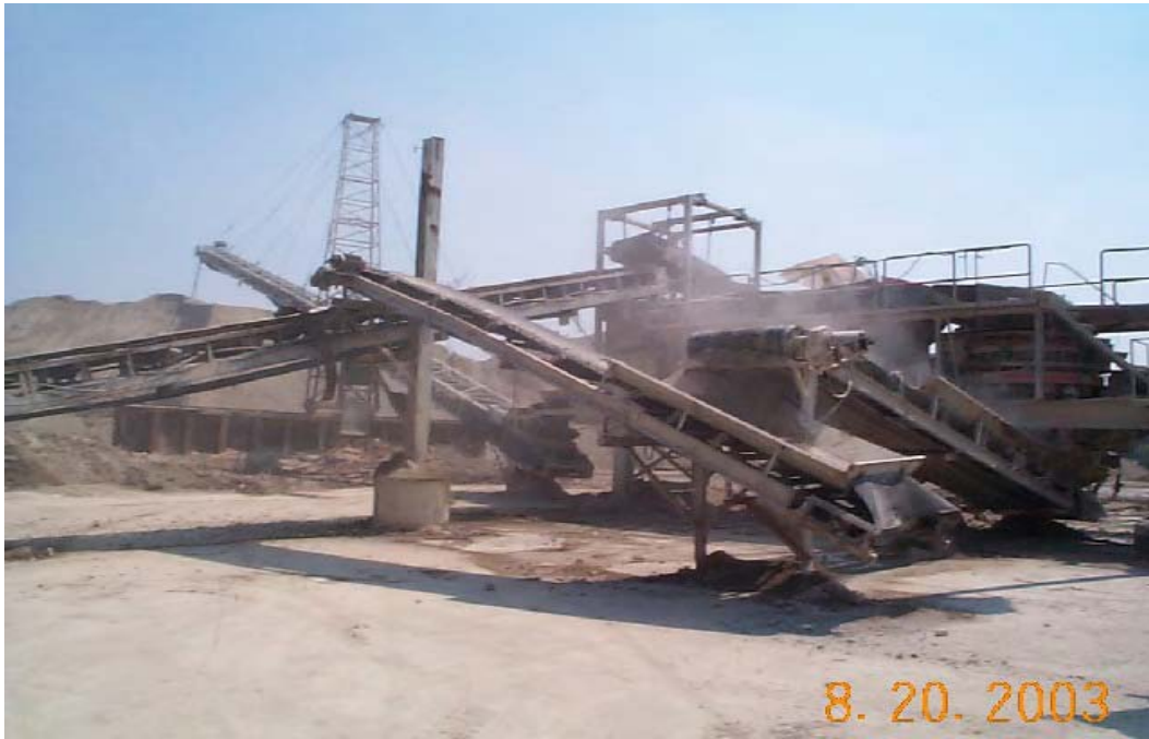
Figure 11. Vibrator feeder, sorting Screen, and Secondary Crusher. Iafrate Crushing Plant Visit. Taylor, MI
