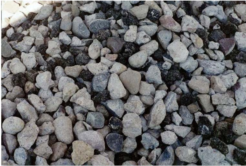
Figure 6.1. Aggregate Base. Stockpile on I-94 Project in Minnesota
