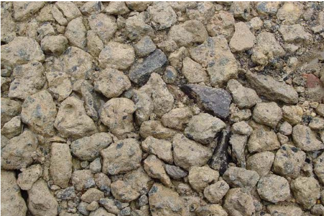
Figure 4. Recycled Concrete Aggregate (RCA). Luck Stone Aggregate Plant. Fairfax, VA
