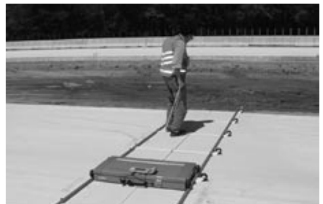
Figure 3. Pulling MIT Scan-2 along the joint being scanned.
