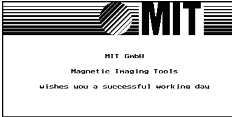
Figure A5. IT2000 display at power-up, when the sensors and communication link between IT2000 and the scan unit are working properly.
