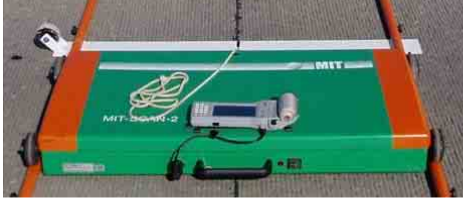
Figure 1. MIT Scan-2, consisting of the sensor unit (a rectangular, green box), onboard computer, and glass-fiber-reinforced plastic rail system.
