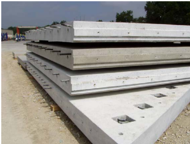
Figure 21. Photo. Precast panels stored at the fabrication plant.
