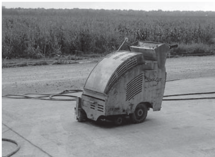
Figure 3. Early-entry saw (Rasouliau, Titi, and Martinez 2006).
