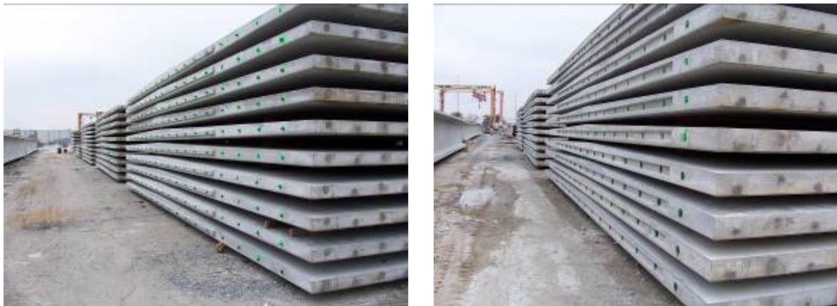
Figure 11. Photo. Discontinuous keyways are shown for the precast panels in storage at the fabrication plant.
