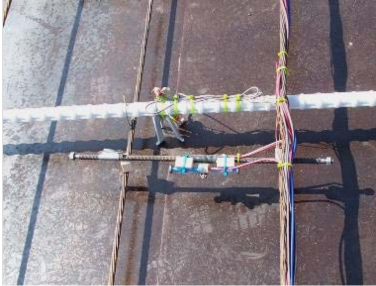
Figure 57. Photo. Instrumented rebar and vibrating wire strain gages for measuring concrete strain.
