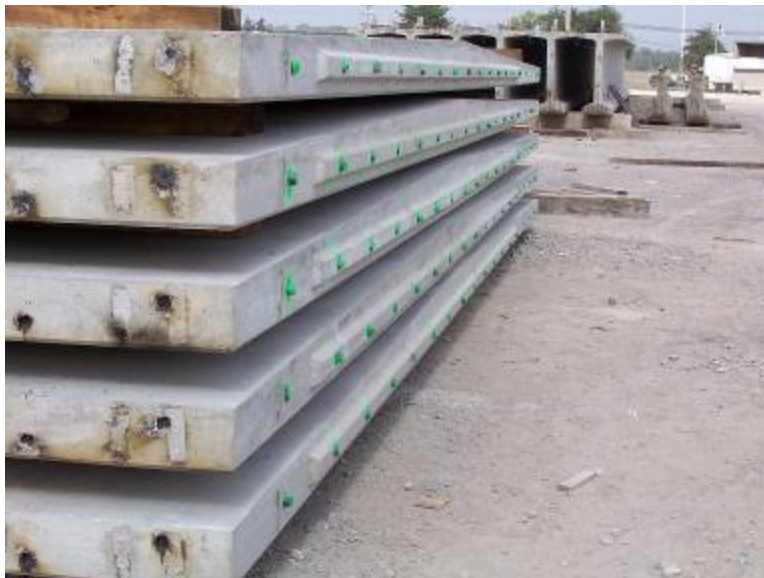
Figure 8. Photo. Precast panels at the fabrication plant after removal from the forms showing the variable thickness cross-section.
