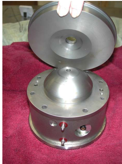
Figure 15. The Hot mix Simulator (HMS) Attachment to the Dynamic Angle Validator (DAV)
