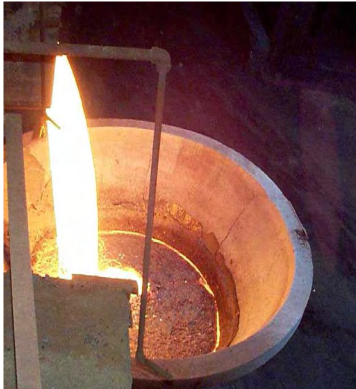
Figure 5. Tapped molten blast furnace slag being directed into ladles at the Ford Rouge River Complex near Detroit, Michigan.
