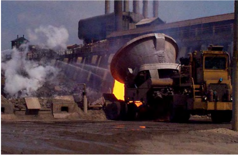
Figure 6. Ladle containing molten blast furnace slag being dumped into a cooling pit at the Ford Rouge River Complex. Note water being sprayed onto the surface. (From Hammerling 1999, p. 14, figure 2.6. © D. M. Hammerling 1999. Reprinted with permission.)
