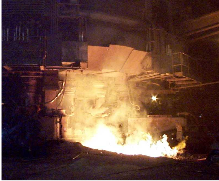
Figure 4. Molten blast furnace slab being tapped at the blast furnace at the Ford Rouge River Complex near Detroit, Michigan.
