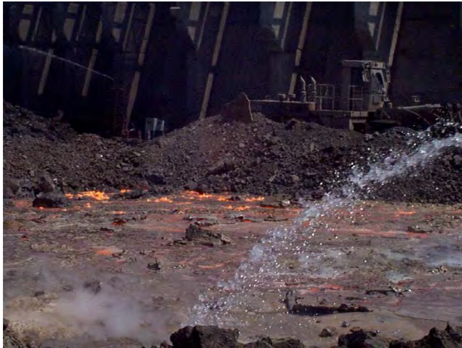
Figure 7. Surface of slag pit at the Ford Rouge River Complex. Note the crushed ACBFS in background and water being sprayed in the foreground to cool the recently molten surface.
