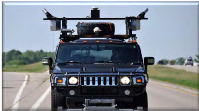
Figure 3.2 Automated Multi-Function Vehicle Used for Pavement Condition Evaluation
