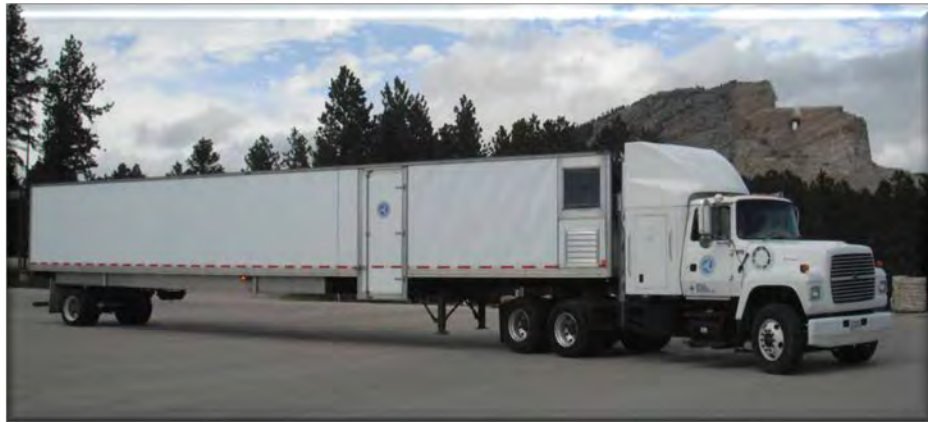
Figure 3.3 Rolling Wheel Deflectometer Used for Structural Evaluation
