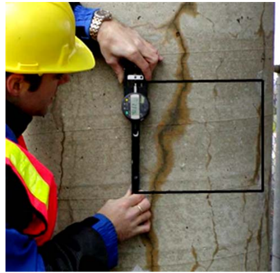
Figure 7.6. In-situ measurements of expansion of ASR-affected concrete elements
