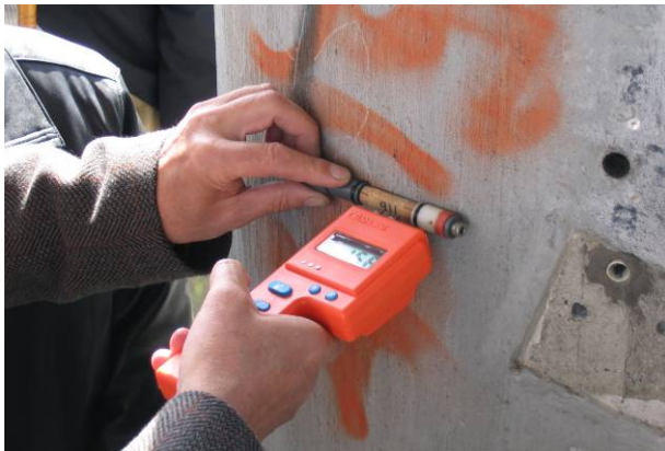
Figure 7.7. In-situ measurements of humidity in concrete. A. Wooden-stick method. B. Vaisala probes.
