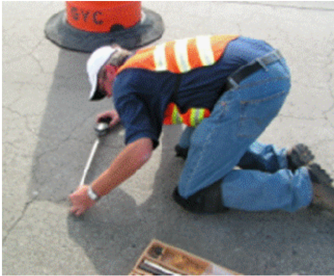
Figure 7.6. In-situ measurements of expansion of ASR-affected concrete elements
