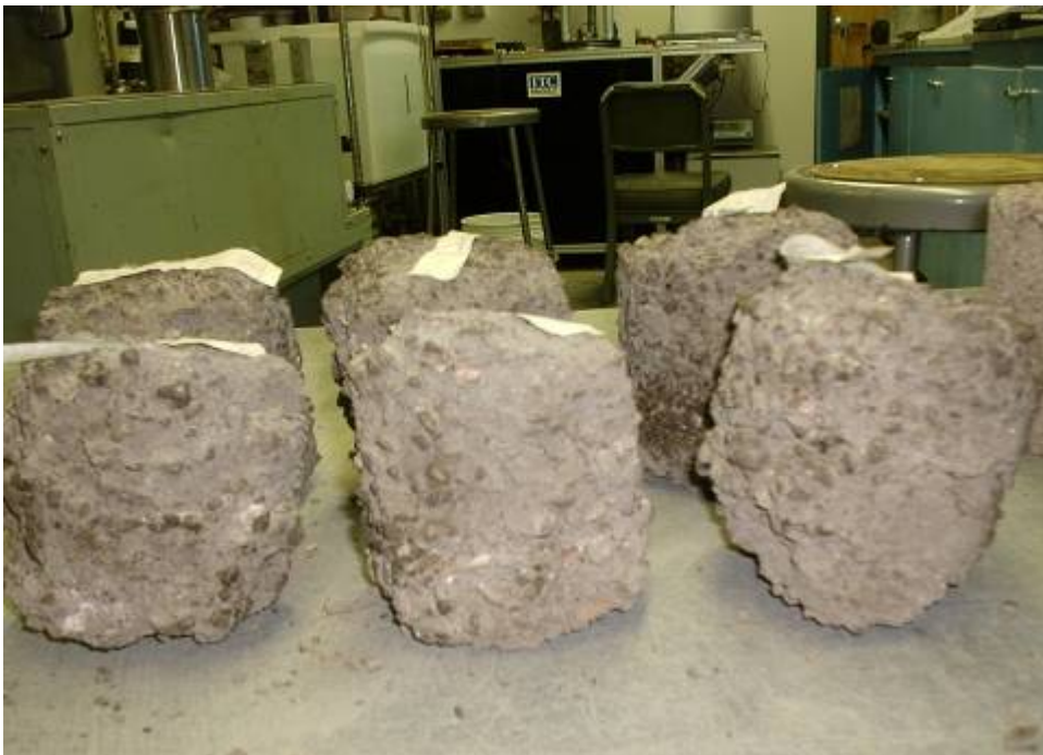
Figure 24: Good Clean material with 50% RAP and 12% FA after 12 cycles.
