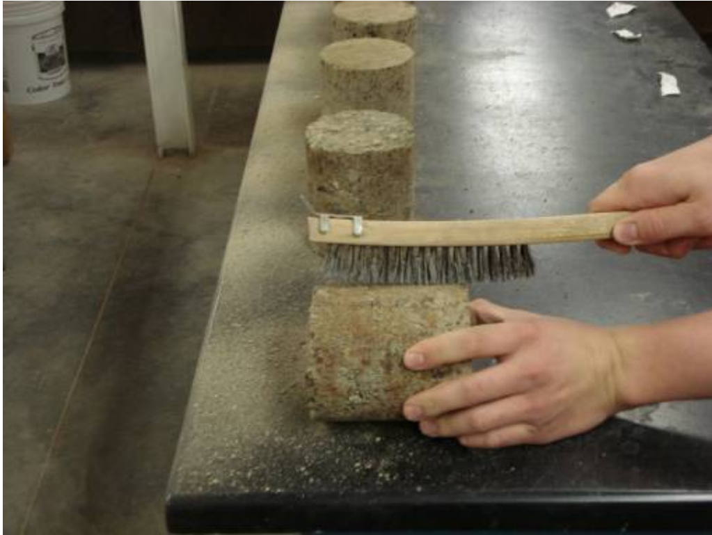
Figure 22: Samples being wire brushed 18 to 20 times on the sides.
