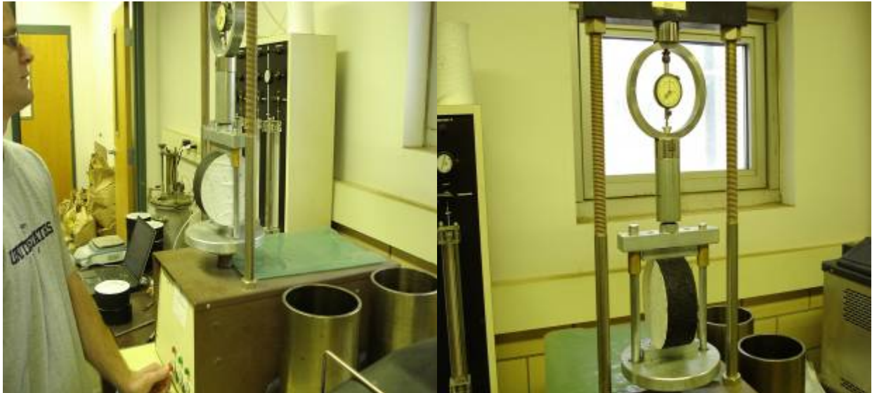
Figure 31: Indirect tensile strength (ITS) testing setup.
