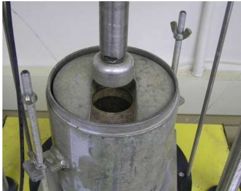
Figure 14: CBR with loading piston being lowered into test specimen.
