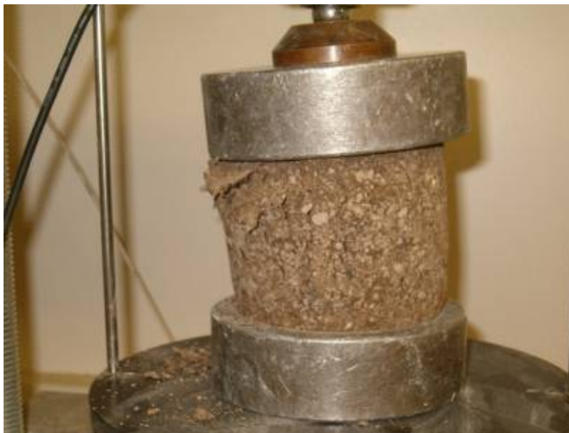
Figure 16: Breaking of the unconfined compression samples.
