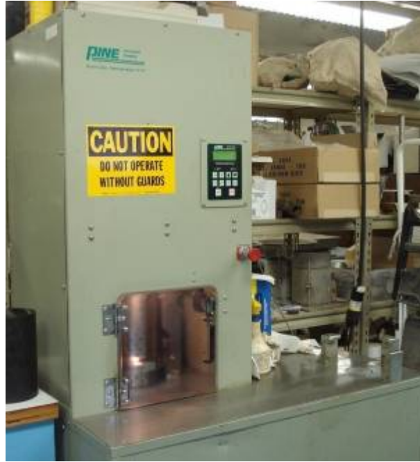
Figure 27: Slotted mold and sample placed in the SGC.
