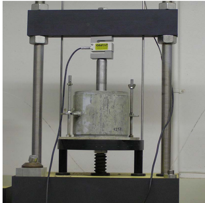
Figure 13: CBR sample in loading frame.
