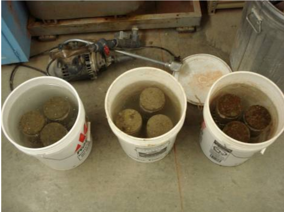
Figure 23: Samples being soaked between the wire brush cycles.
