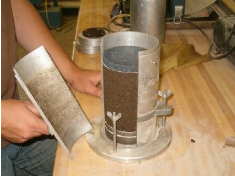
Figure 5: Removing the sides of the mold.
