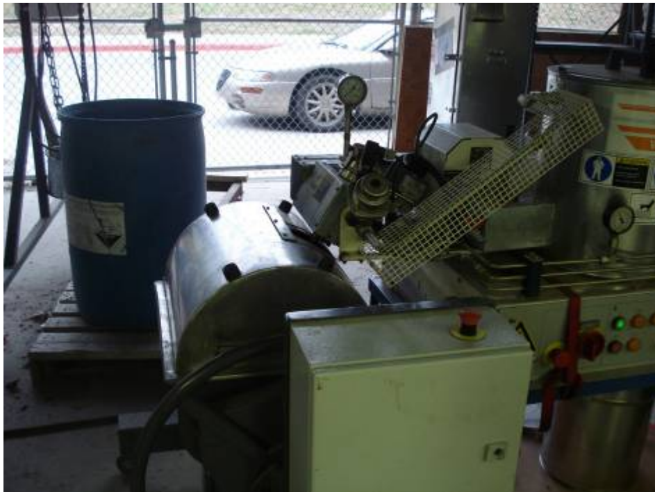
Figure 34: Asphalt binder foaming machine with pugmill mixer.
