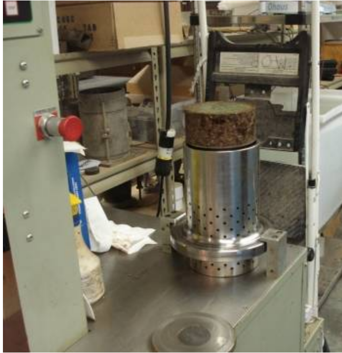
Figure 26: Gyratory compactor with sample in the mold carriage.
