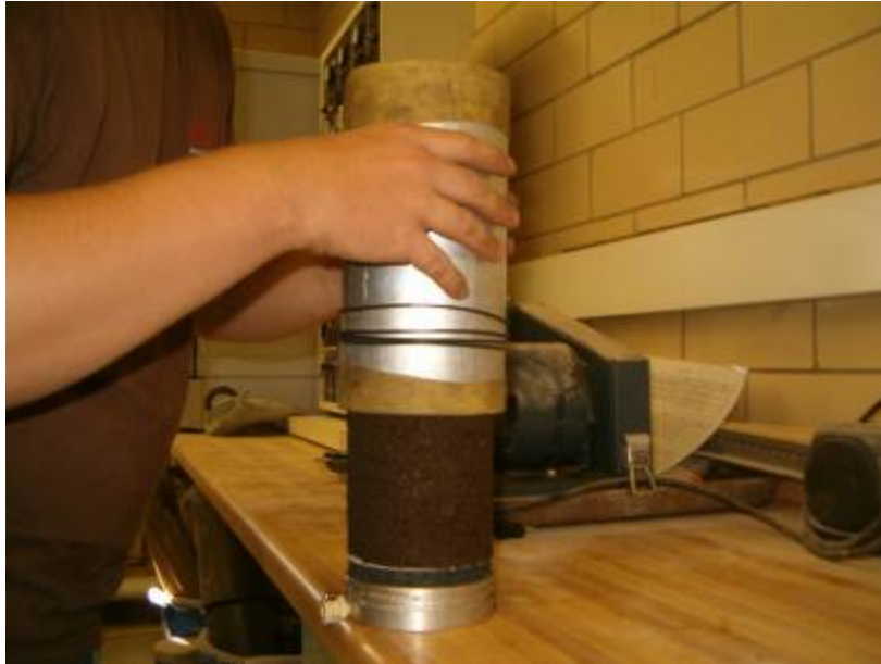
Figure 9: Placing the membrane on the sample.
