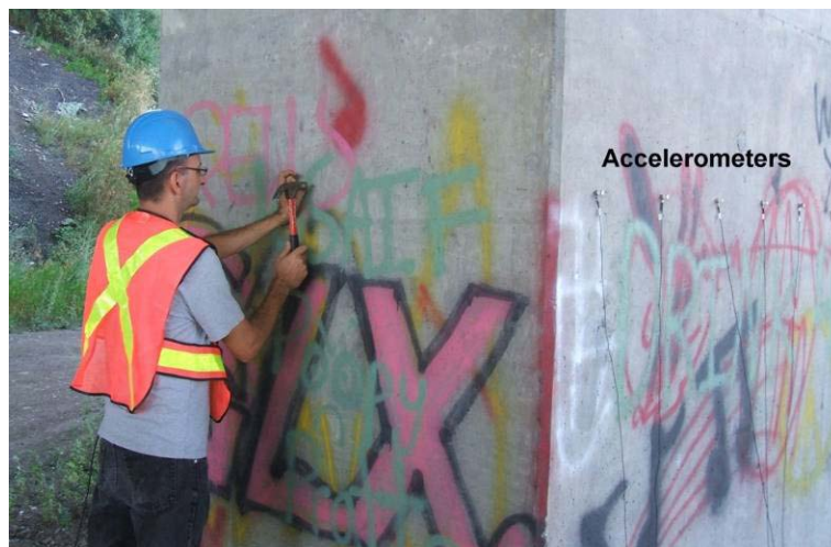
Figure 76. Seismic tomography on Column 1 of the I-395 bridge over the Penobscot River.
