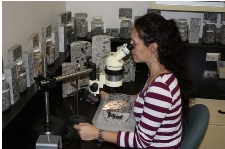
Figure 3. Examination of a polished concrete section under the stereomicroscope for the determination of the Damage Rating Index.
