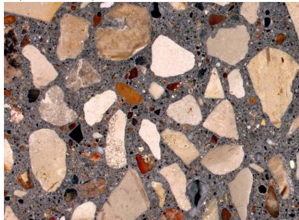
Figure 174. Typical micrographs of the polished core sections showing carbonate (mainly) and chert coarse aggregate particles ( \frac{3}{4} inch [2 cm] nominal size) in a dark grey cementitious matrix. There is no visible evidence of cracking both in the aggregate particles (coarse and fine) as well as in the cementitious matrix at the magnification used for the DRI (16x).
