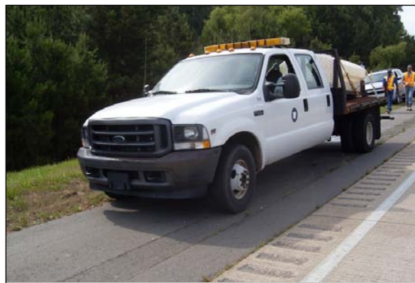
Figure 49. Photograph of AHTD maintenance truck, equipped with truck-mounted, tank sprayer. The truck/sprayer was pre-calibrated in order to deliver the target application rate of 3.1 m 2 /L (125 ft 2 /gal).
