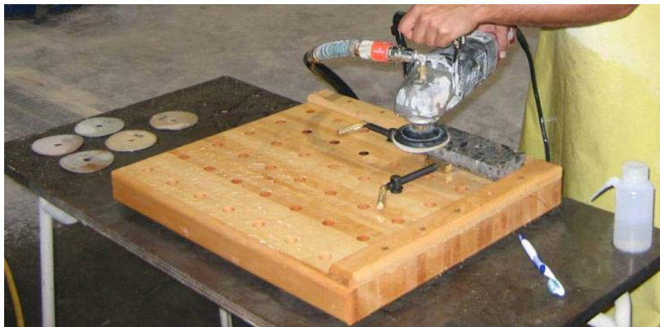
Figure 1. Polishing process of the concrete specimens for the Damage Rating Index.
