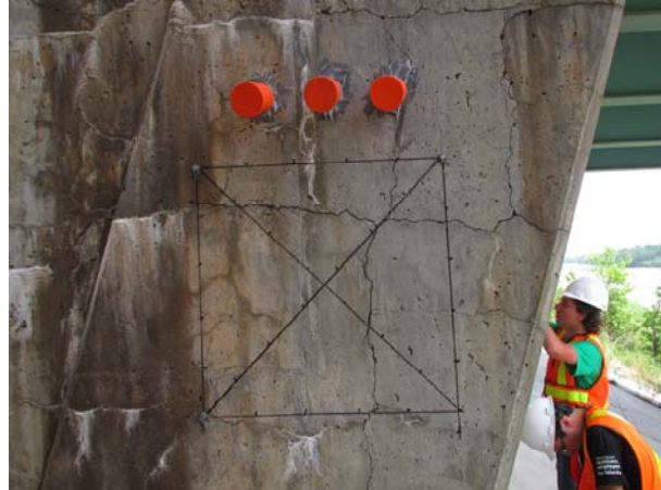
Figure 15. Sleeves and stoppers used for humidity measurements, inserted into three holes drilled at different depths into the selected concrete element.
