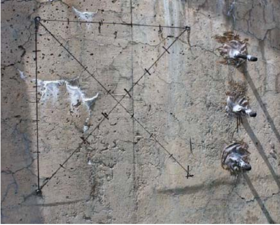
Figure 15. Sleeves and stoppers used for humidity measurements, inserted into three holes drilled at different depths into the selected concrete element.
