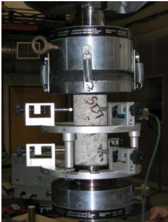
Figure 6. Setup used for the Stiffness Damage Test (SDT).
