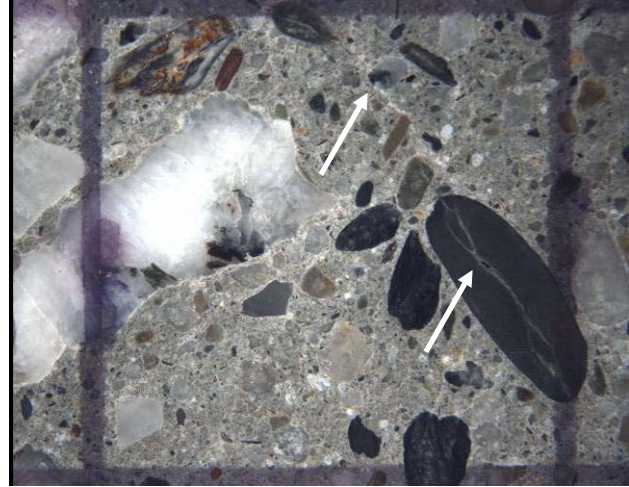
Figure 240. Polished concrete surfaces (cores extracted from the barrier walls of two bridges carrying interstate I-89 over Dog River near Montpelier, VT).
