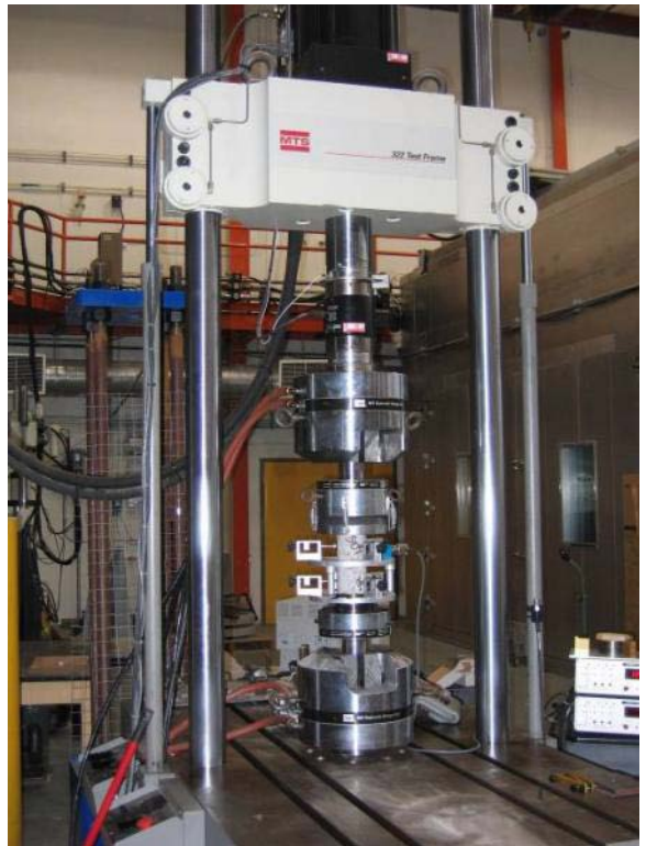
Figure 6. Setup used for the Stiffness Damage Test (SDT).
