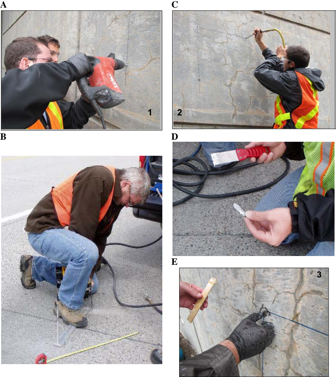
Figure 8. Embedding steel pins for expansion measurements. A&B: Drilling of the holes at the corners of the 500-mm (20-in.) grid (or crack map). C: Cleaning excess drilling debris with compressed air. D: Epoxy spread along the steel pin. E: Inserting the steel pin into the hole, flush with the surface of the concrete.
