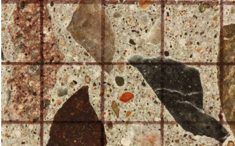
Figure 2. One cm by one cm (0.4 by 0.4 in.) grid drawn on the surface of a polished concrete section for petrographic examination using the DRI method.
