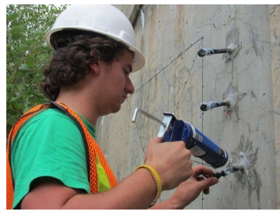
Figure 18. A-C: In-situ humidity and temperature measurements. D: Sealing of the plastic sleeve using the rubber plug with silicone.
