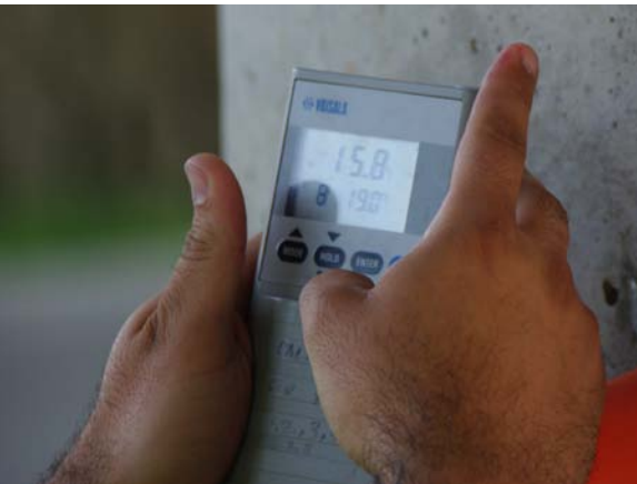
Figure 18. A-C: In-situ humidity and temperature measurements. D: Sealing of the plastic sleeve using the rubber plug with silicone.
