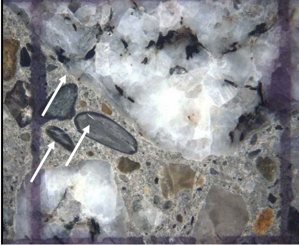
Figure 240. Polished concrete surfaces (cores extracted from the barrier walls of two bridges carrying interstate I-89 over Dog River near Montpelier, VT).
