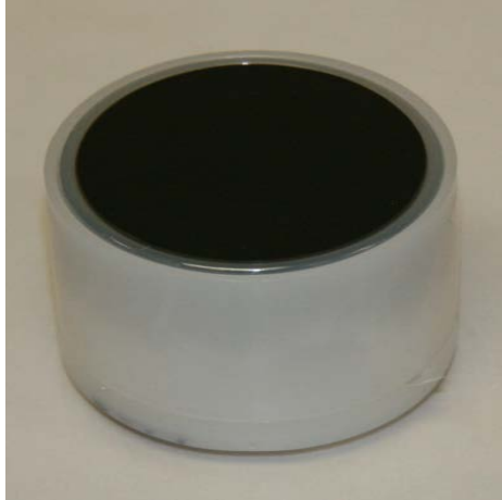
Figure 2. Photo. XRF cup (inverted) filled with asphalt.
