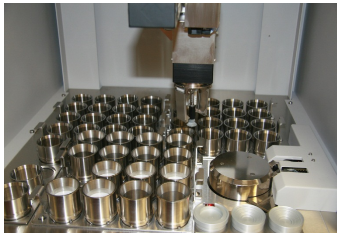
Figure 4. Photo. Interior of XRF spectrometer.
