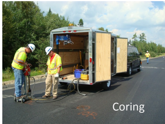
Figure 21. Typical spot tests and coring for an IC field site
