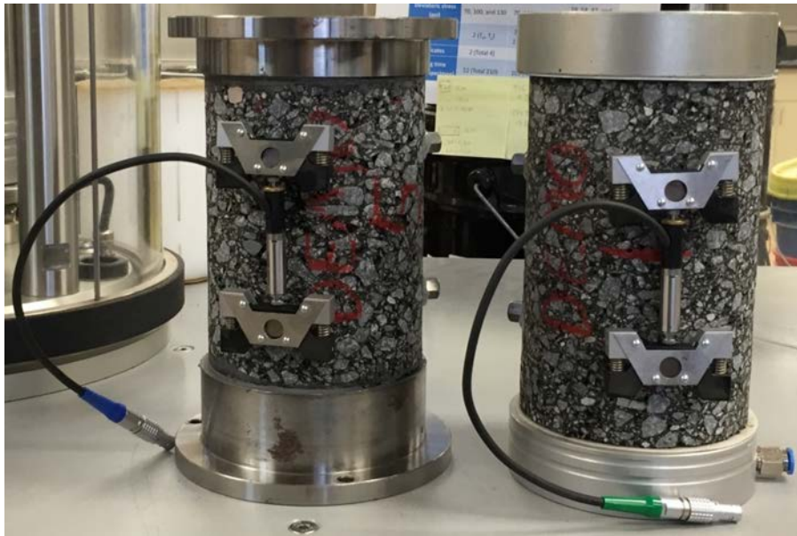
Figure 2. Typical AMPT Cyclic Fatigue specimen (left) alongside dynamic modulus specimen (right).
