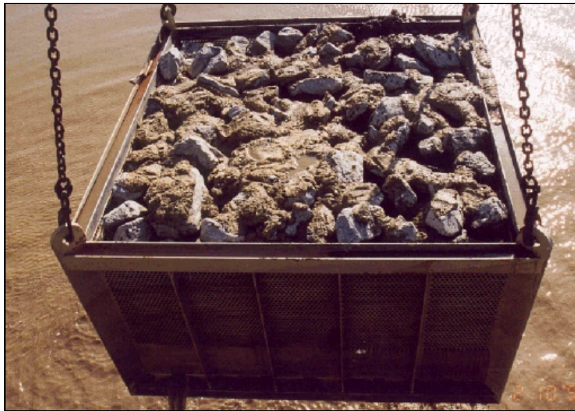
Figure 12.21. Test box used during underwater grout placement.
