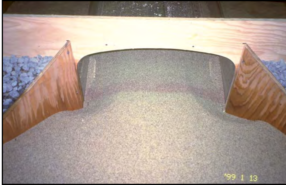
Figure 18.5. Arched model with wing walls (Kerenyi et al. 2003).
