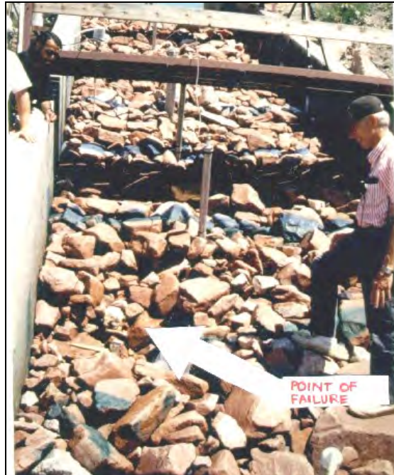
Figure 5.7. Riprap failure in 1994 tests ( d_{50} = 1.27 ft (386 mm))
