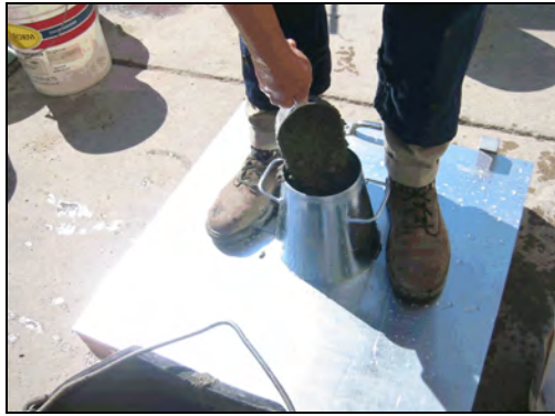
a. Slump cone and test table
