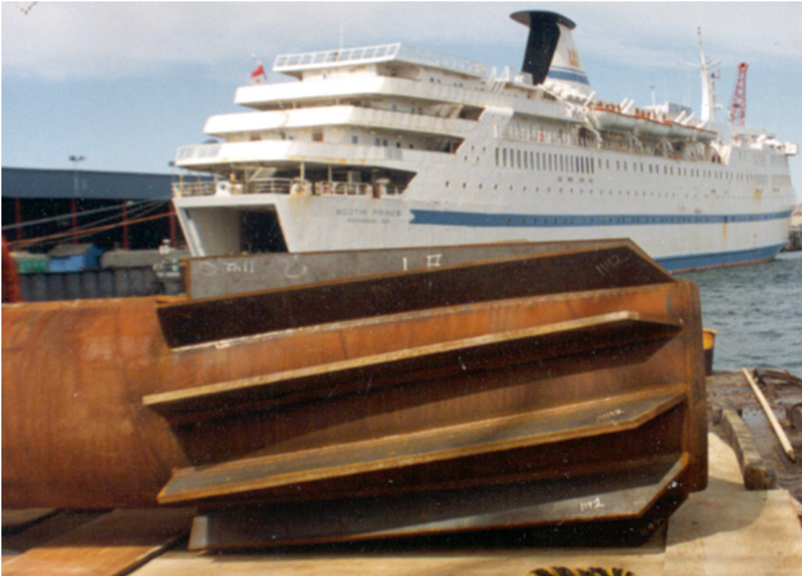
Figure 6-19 30 inch diameter Spin Fin pile.
