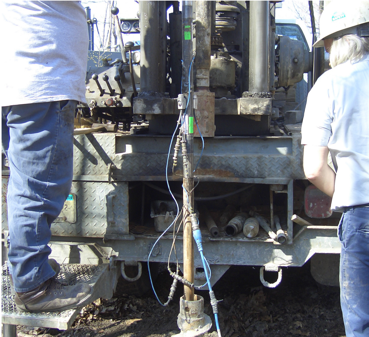
Figure 5-4 Instrumented 2 foot long AW rod atop drill string for SPT hammer energy measurements.
