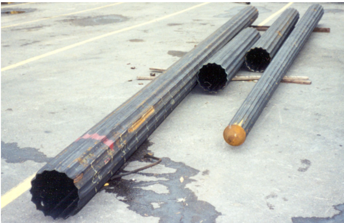
Figure 6-16 Tapered Monotube section (right) with add-on sections (left).
