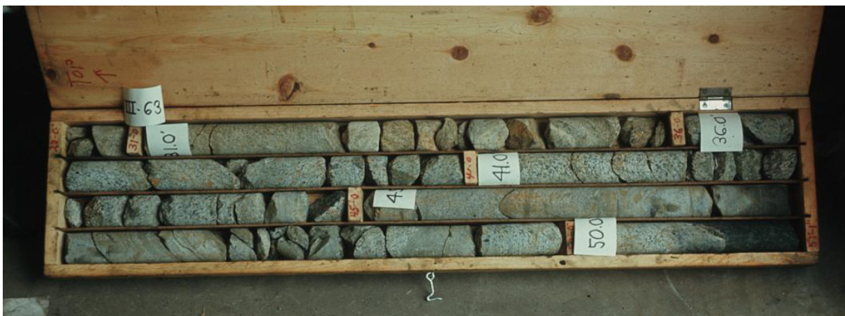
Figure 4-4 Rock core samples.
