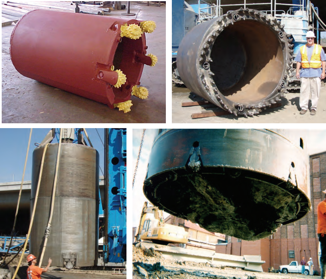
Figure 5-24 Double Wall Core Barrels
