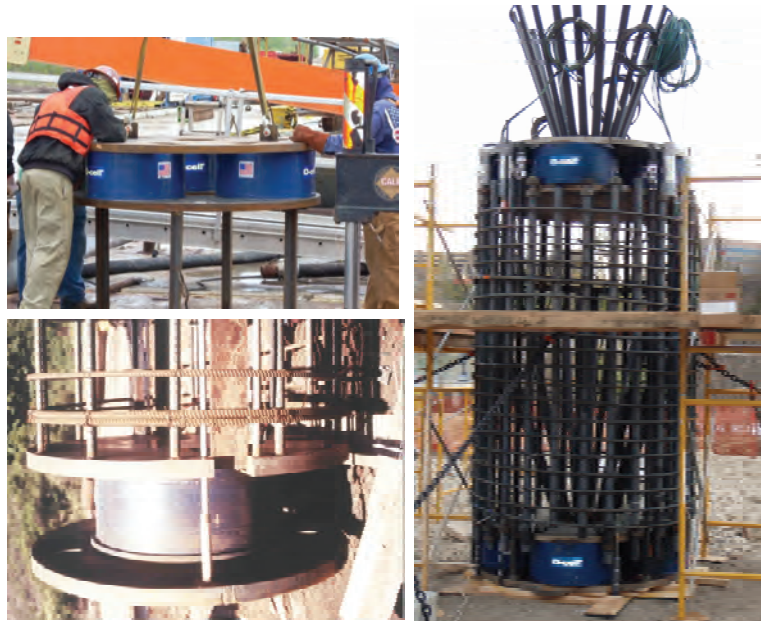
Figure 17-16 Single O-Cell (bottom left), Multiple O-Cell Assembly (top left) and Multi-Level O-Cell Assembly (right)
