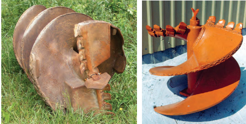
Figure 5-16 Double Flight Earth Augers
