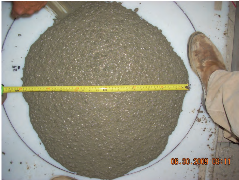
Figure A-13 Slump Flow Measurement on High-Performance Concrete of Design Example (Photo courtesy of Paul Axtell)
