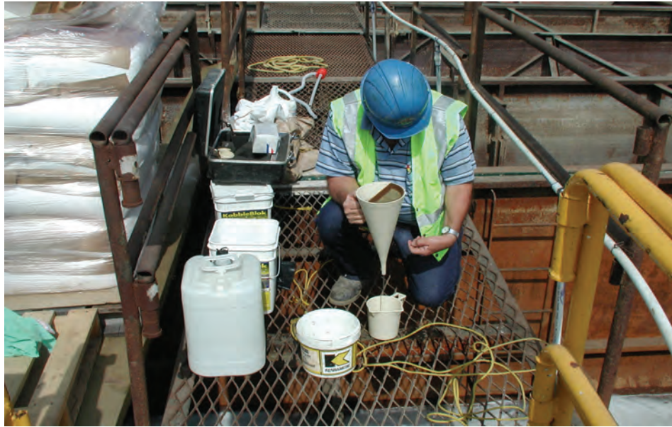
Figure 7-10 Marsh Funnel Test for Field Evaluation of Slurry Viscosity
