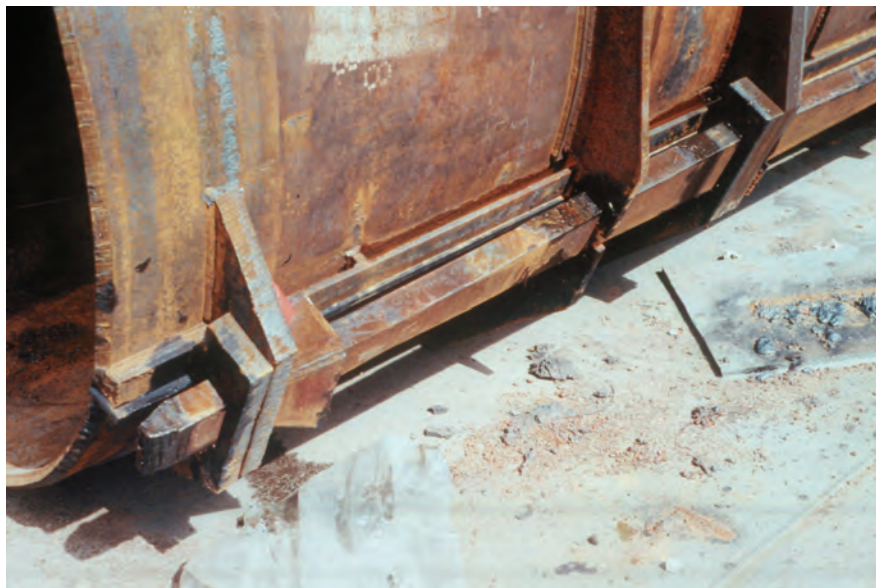
Figure 6-12 Locking Mechanism for a Removable Casing
