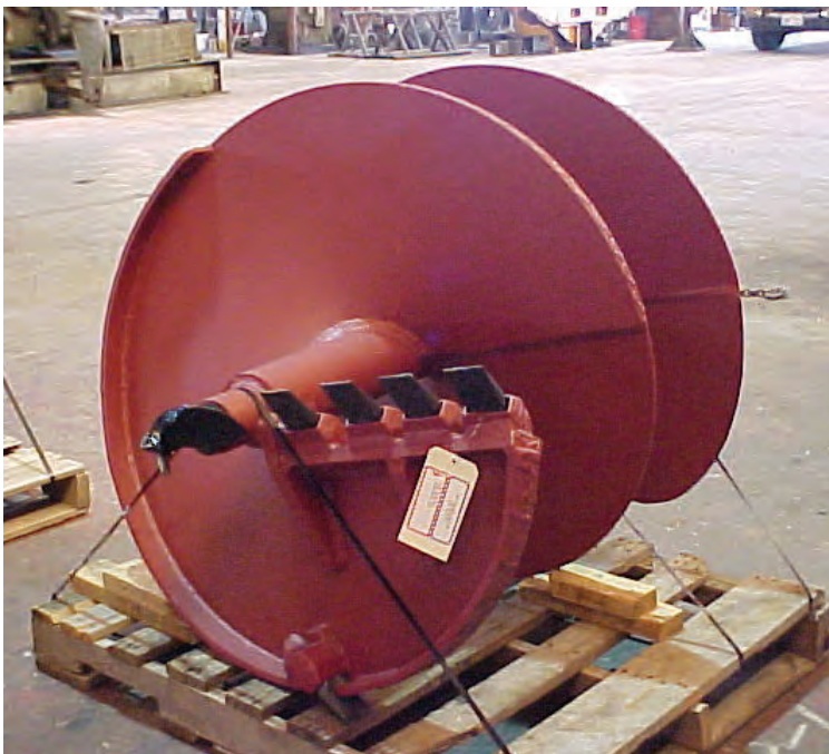
Figure 5-15 Single Flight Earth Augers
