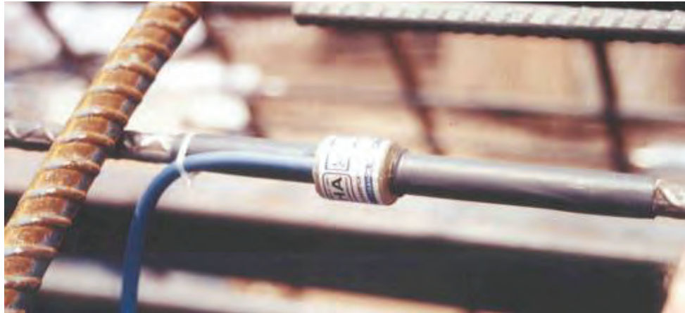
Figure 17-50 Vibrating Wire Type Strain Gauge
