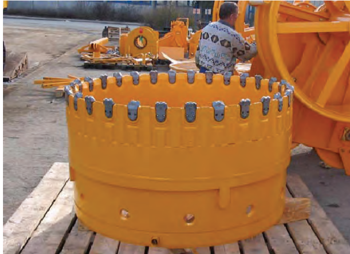
Figure 6-9 Cutting Shoe for Segmental Casing
