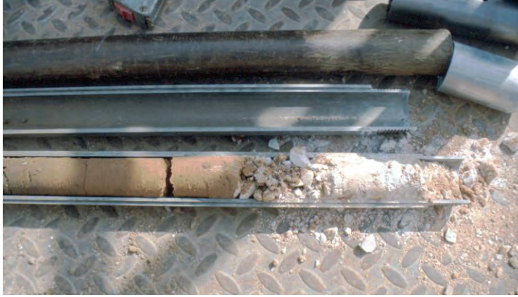
Figure 3-2 Split-Spoon Sampler for Determination of Soil Stratigraphy
