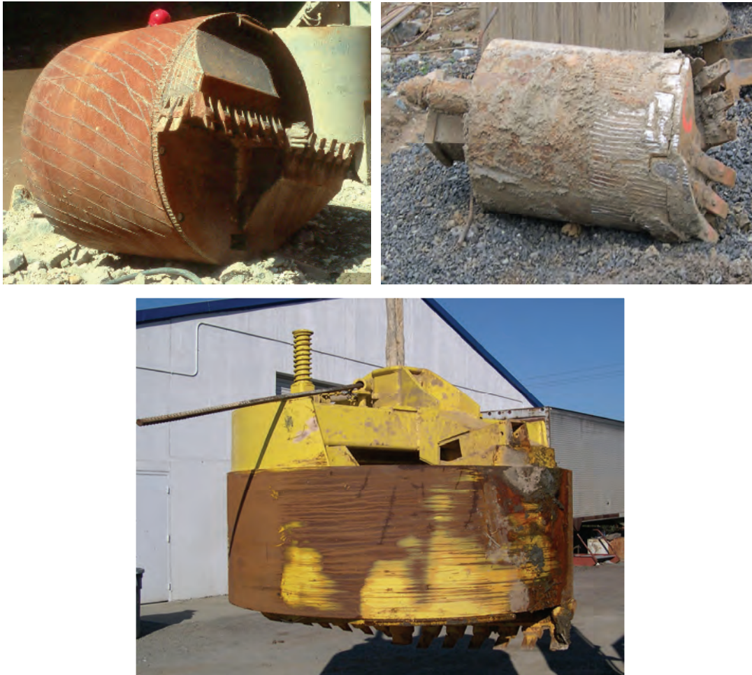
Figure 5-21 Typical Drilling Buckets
