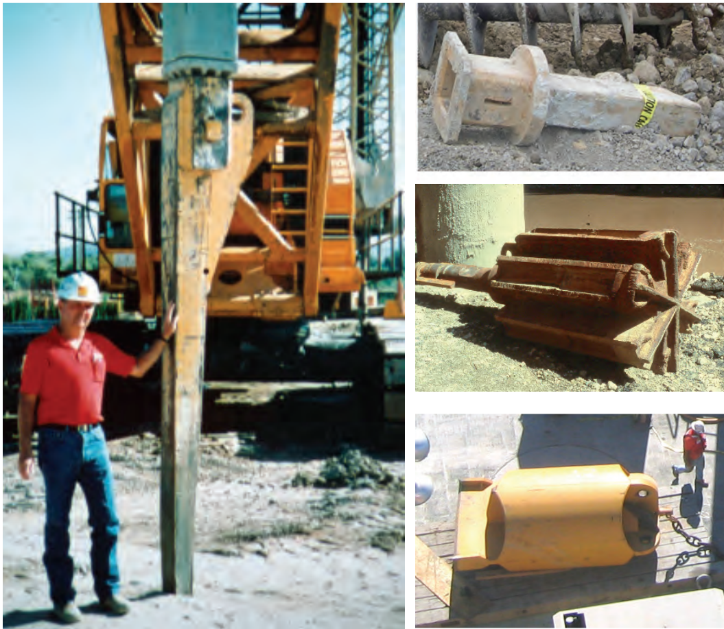
Figure 5-32 Drop Chisels and Rock Breakers
