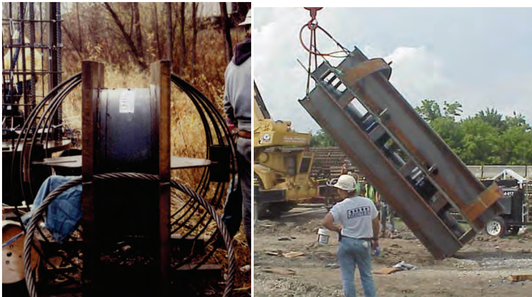
Figure 17-59 Bi-directional Lateral Testing Apparatus Using Embedded O-cells
