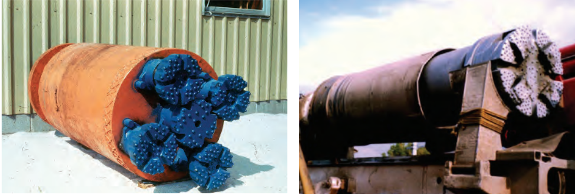
Figure 5-33 Downhole Impact Hammers
