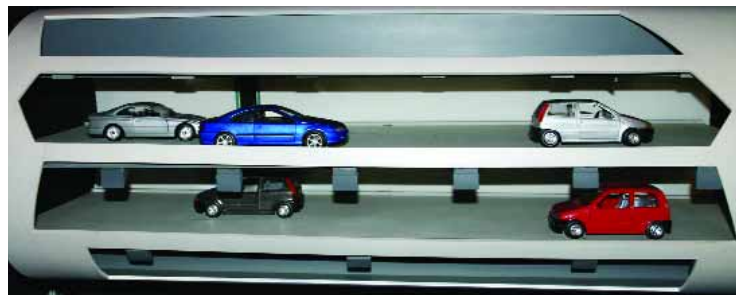
Figure 9. Model of A86 twin roadway tube. Top: full-size model of one section. Bottom: scale model of twin tube.
