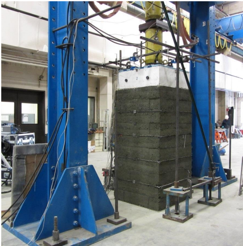
Figure 21. Photo. TF-10 PT setup with reaction frame.
