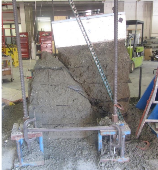
Figure 36. Photo. TF-13 at failure with S_v = 11\frac{1}{4} inches, T_f = 3,600 lb/ft, and 21A material.
