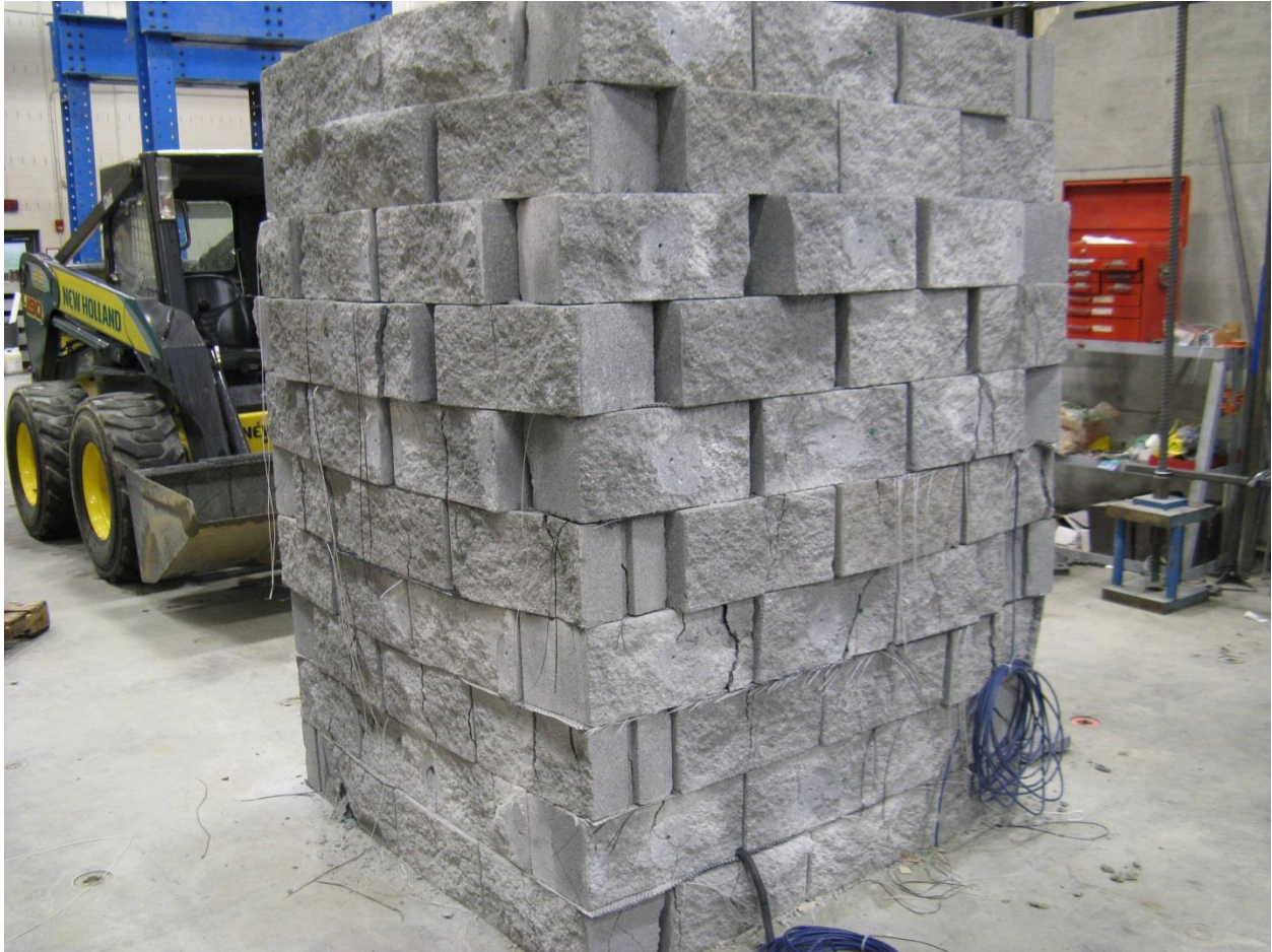
Figure 39. Photo. Post-test picture of TF-6 ( S_v = 7\frac{5}{8} inches, T_f = 4,800 lb/ft).
