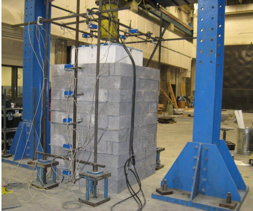
Figure 20. Photo. TF-6 PT setup with reaction frame.
