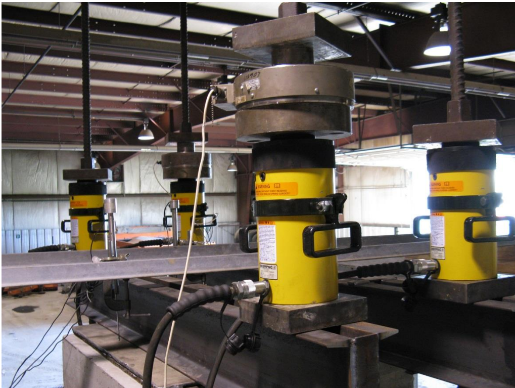
Figure 18. Photo. Hollow core hydraulic jacks for PT assembly.
