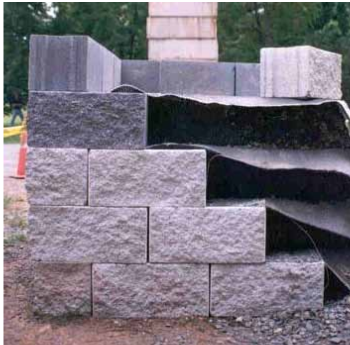
Figure 6. Photo. Cut-away of GRS mass.
