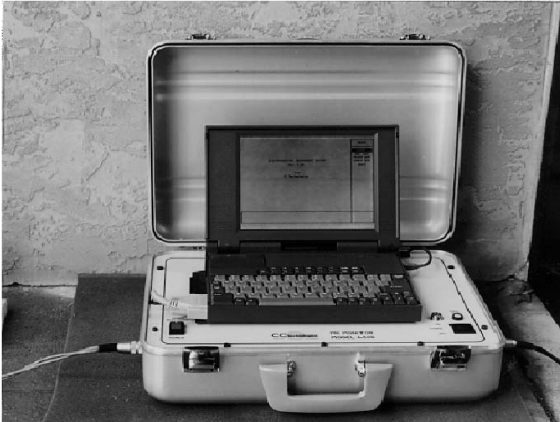
Figure 3-9. Automated polarization resistance measurement equipment.
