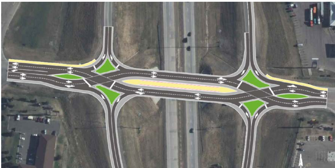
Figure 4. Photo. Four-lane DDI configuration.
