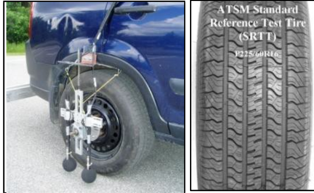
Figure 19. OBSI dual probe system and the SRTT.
