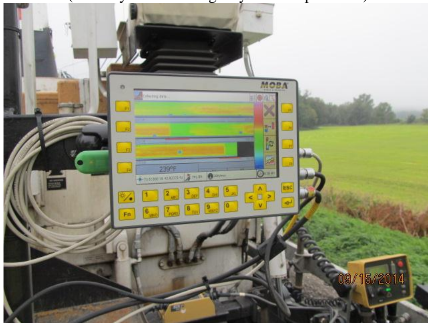
Figure 8. Photo. Interface controller attached to the rear of the paver for real-time monitoring. (courtesy: Vermont Agency of Transportation)
