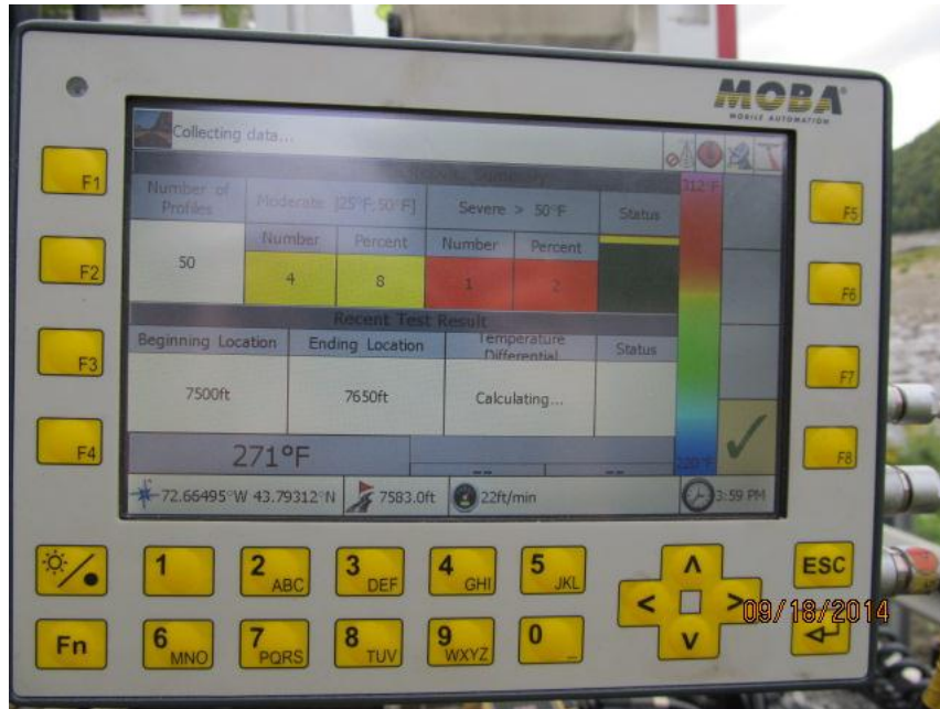
Figure 9. Photo. Interface controller monitor showing number and percentage of moderate and severe thermal profiles in yellow and red boxes. (courtesy: Vermont Agency of Transportation)
