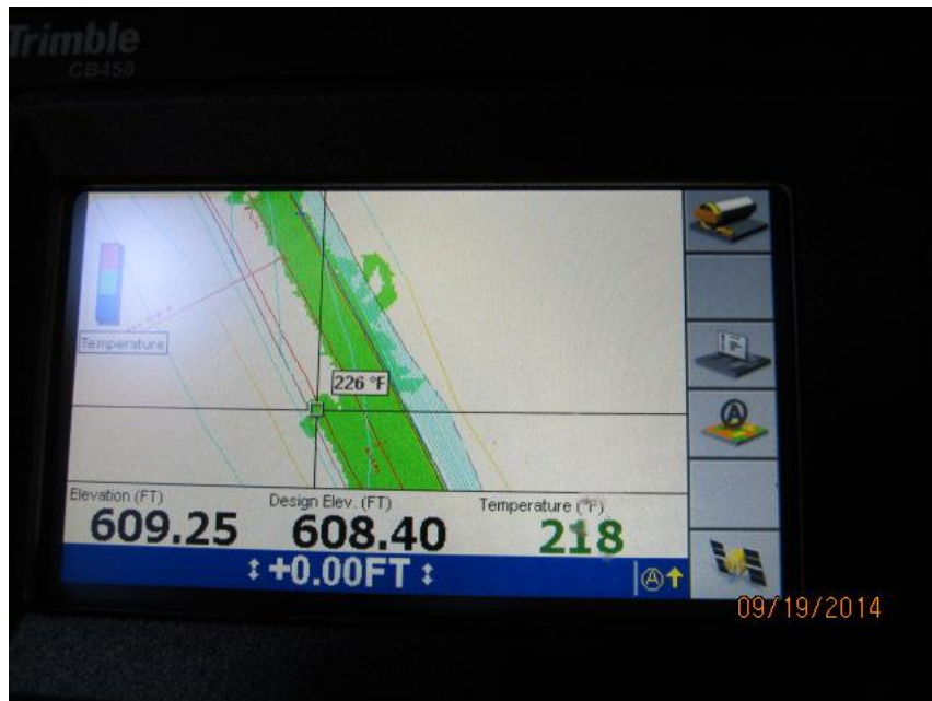
Figure 3. Photo. Temperature map from on-board IC data collector. (courtesy: Vermont Agency of Transportation)
