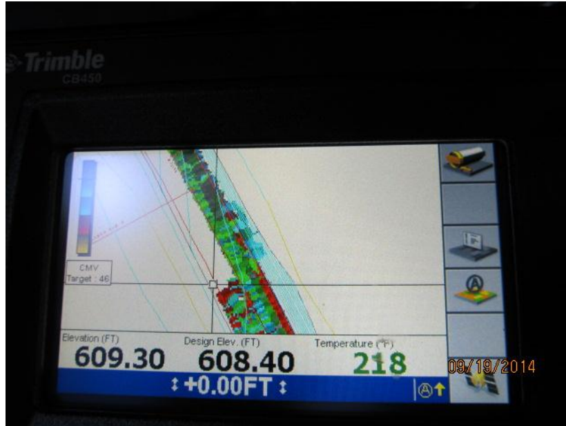
Figure 4. Photo. CMV data screen from on-board data collector. (courtesy: Vermont Agency of Transportation)
