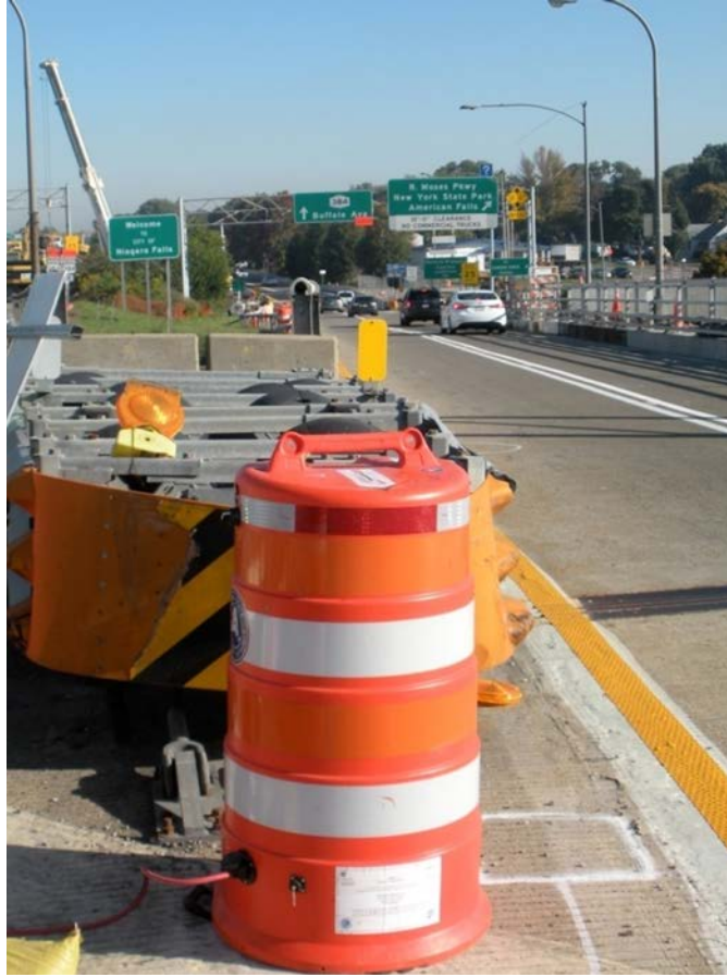
Figure 35. Photo. The iCone® traffic barrel measures speed of diverted traffic.
