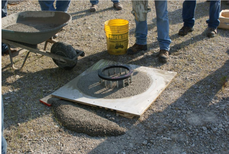
Figure 8. Cage test results of modified slump of self-consolidating concrete.
