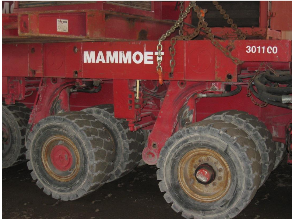
Figure 60. Photo. Close-up of the SMPT wheels. Each pair of wheels is full articulated and is capable of moving independently of the remaining wheels.
