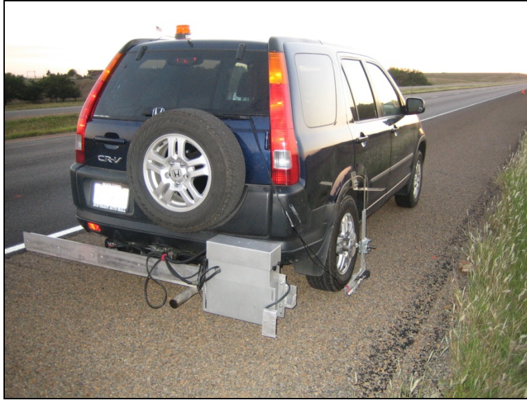
Figure 21. Laser profiler mounted behind the test vehicle.
